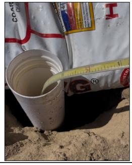
Photograph: 9 Date: 8/4/2025 Description: Dry depth to water boring at  $\sim$ 56' bgs.
