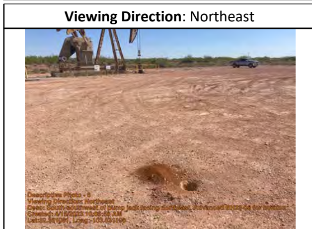
South-southwest of pump jack facing northeast. Advanced BH23-08 for horizontal delineation.
