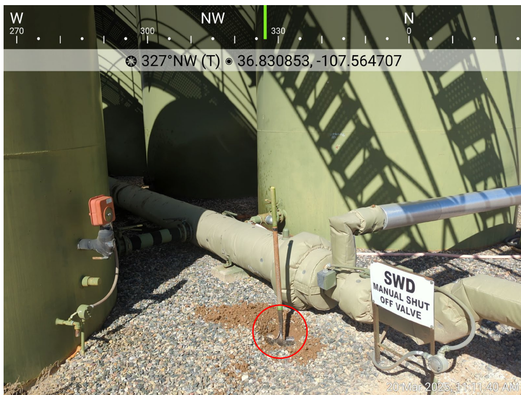
Photo 25: SS24 (0-12") collected as a grab sample for horizontal delineation east of ASTs.
