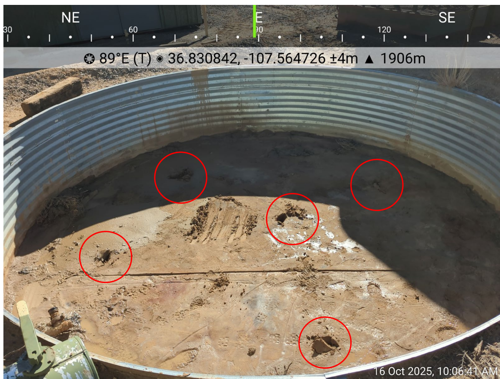
Photo 45: SS45 collected as a five-point composite confirmation sample from the base of the BGT following removal.
