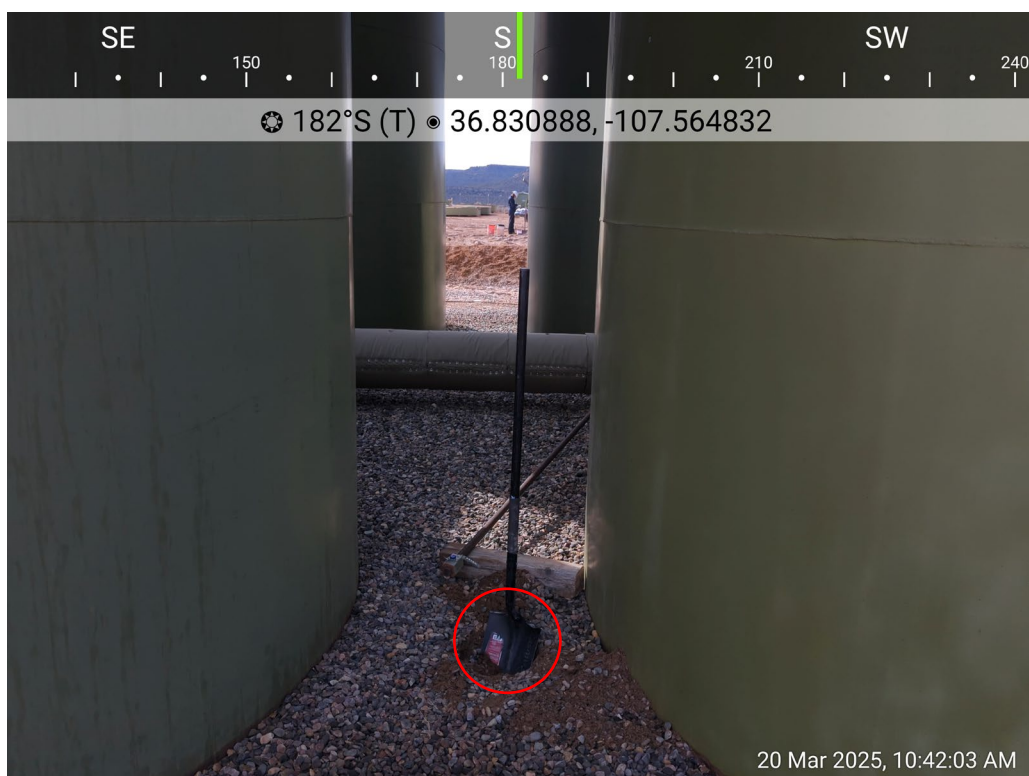
Photo 22: SS21 (0-8") collected as a grab sample for horizontal delineation between northern ASTs.
