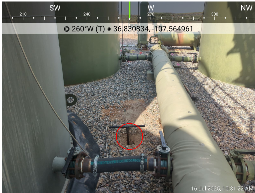
Photo 33: SS33 (0-1'), (1-2'), (2-3'), (3-4'), (4-5'), (5-6'), (6-7'), (7-8'), (8-9'), and (9-10') collected for vertical delineation within the release area.
