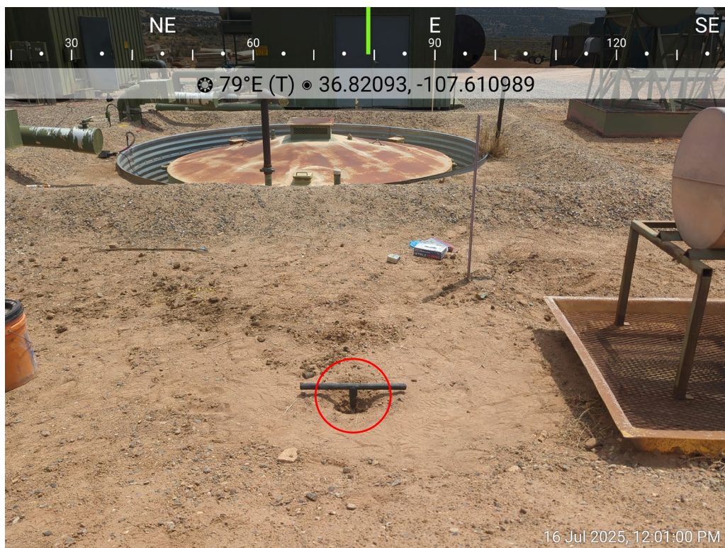
Photo 34: SS34 (1-2'), SS34 (4-5'), SS34 (9-10') collected as vertical delineation samples within the release area.
