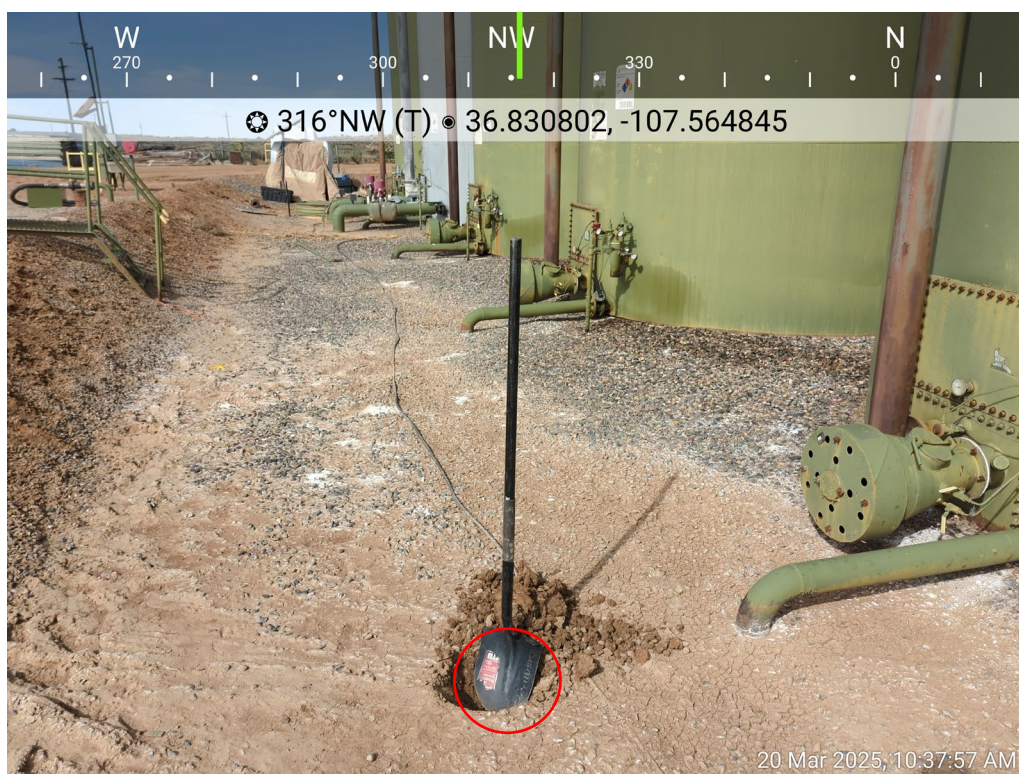
Photo 20: SS19 (0-12") collected as a grab sample for horizontal delineation south of ASTs.
