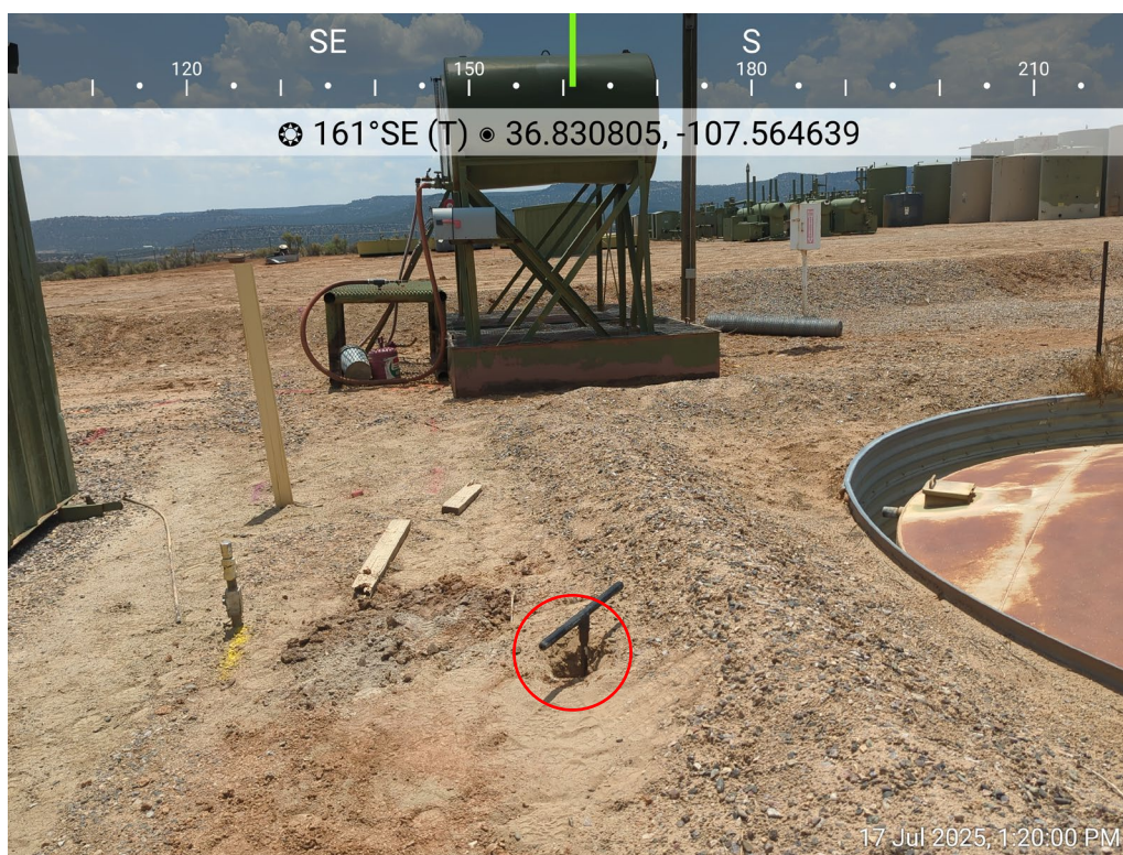
Photo 40: SS40 (1-2'), SS40 (4-5'), SS40 (8-9') collected as vertical delineation samples within the release area.
