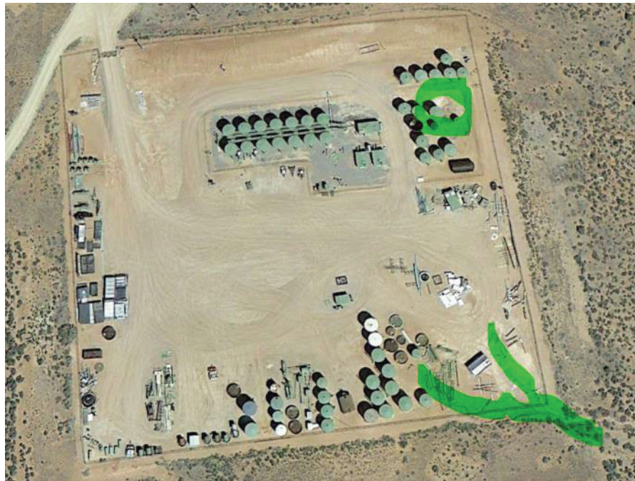
Photo 12: 2013 aerial documenting potential spill in northeast tank storage. This area must be assessed.
