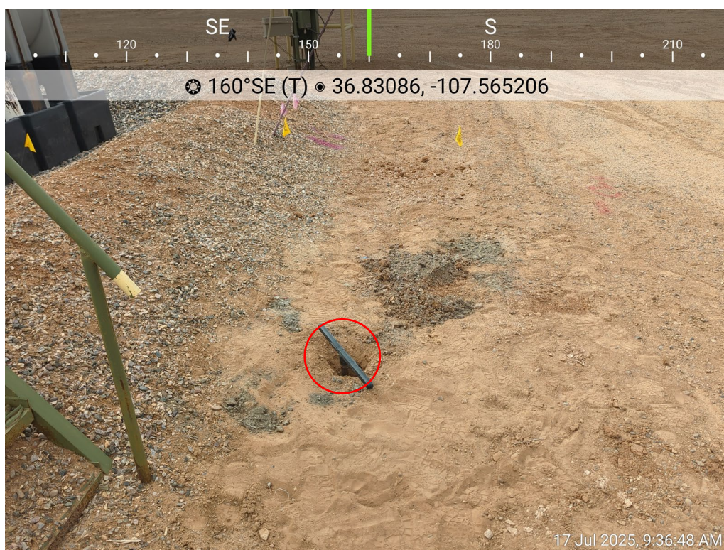
Photo 36: SS36 (1-2'), SS36 (4-5'), SS36 (9-10') collected as vertical delineation samples outside the release area.
