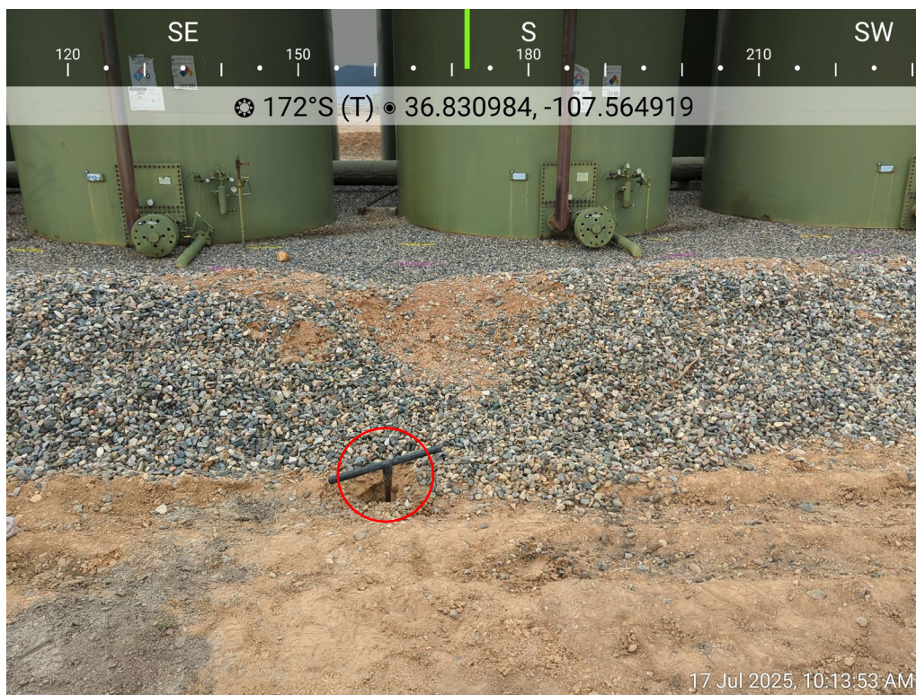
Photo 37: SS37 (1-2'), SS37 (4-5'), SS37 (9-10') collected as vertical delineation samples within the release area.
