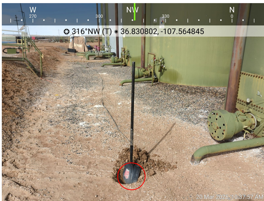
Photo 20: SS19 (0-12") collected as a grab sample for horizontal delineation south of ASTs.
