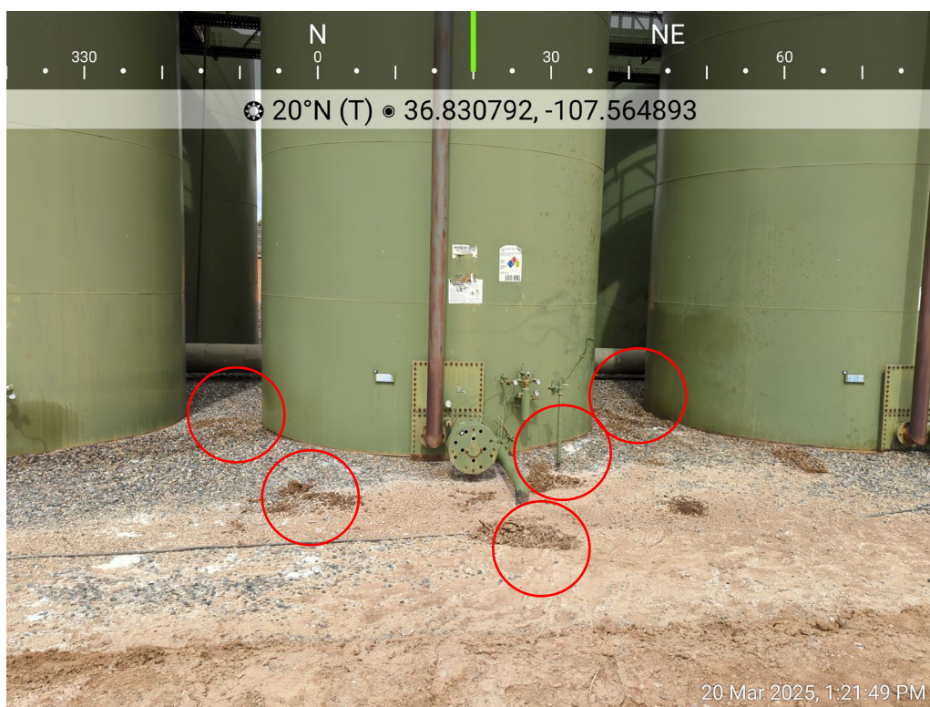
Photo 30: SS30 (0-6") collected as a 5-point composite sample from within the release area.
