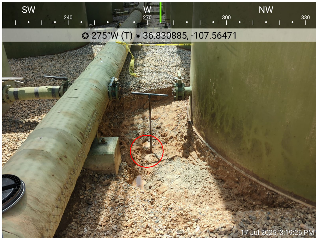
Photo 43: SS43 (2-3'), (3-4'), (4-5'), (5-6'), (6-7'), (7-8'), (8-9'), and (9-10') collected for vertical delineation within the release area.
