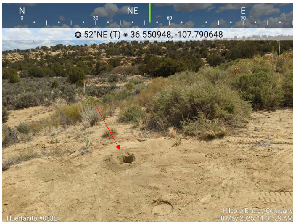
Photo 17: BH-07 (16-18') collected northeast of bermed area. Bore hole backfilled with grout.
