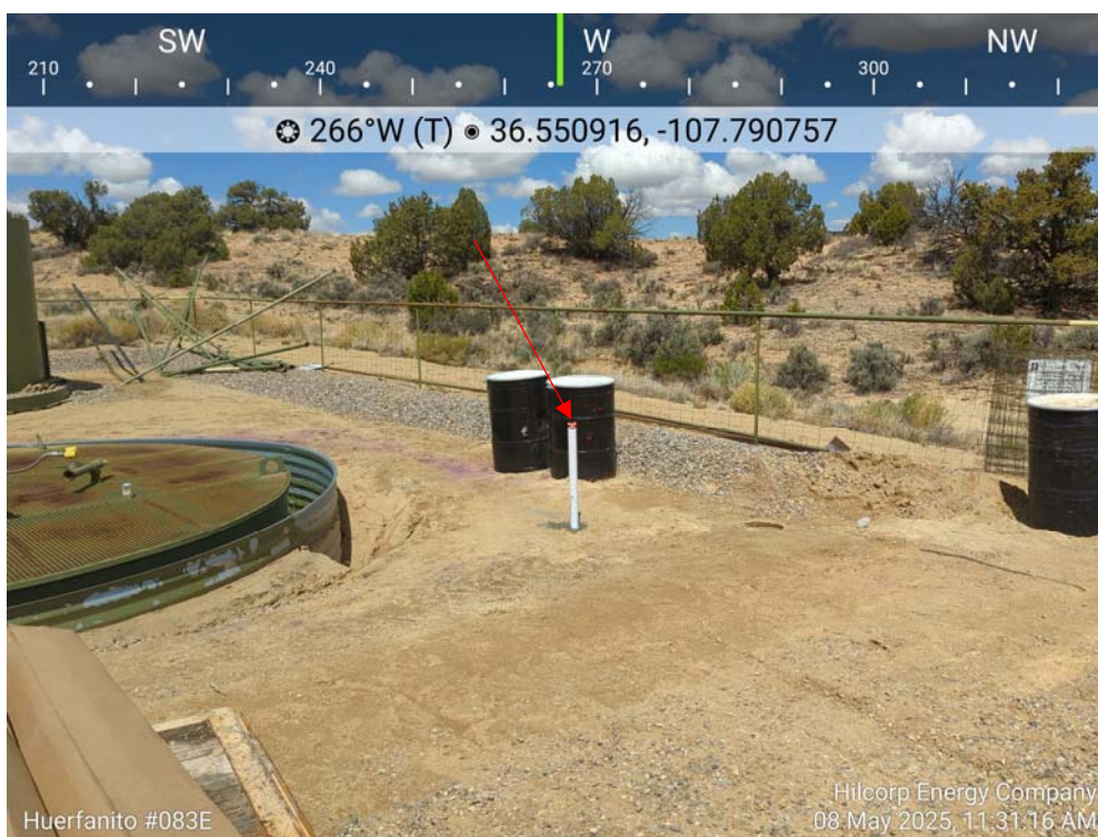
Photo 14: BH-04 (18-20') collected northeast of BGT. Bore hole completed as SVE point SVE-03. Drilled 5/7/2025.
