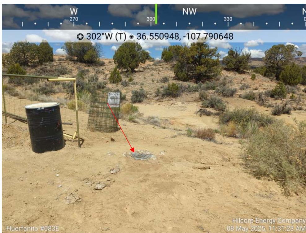
Photo 15: BH-05 (14-16') and BH-06 (18-20') collected northeast of bermed area. Bore hole backfilled with grout.
