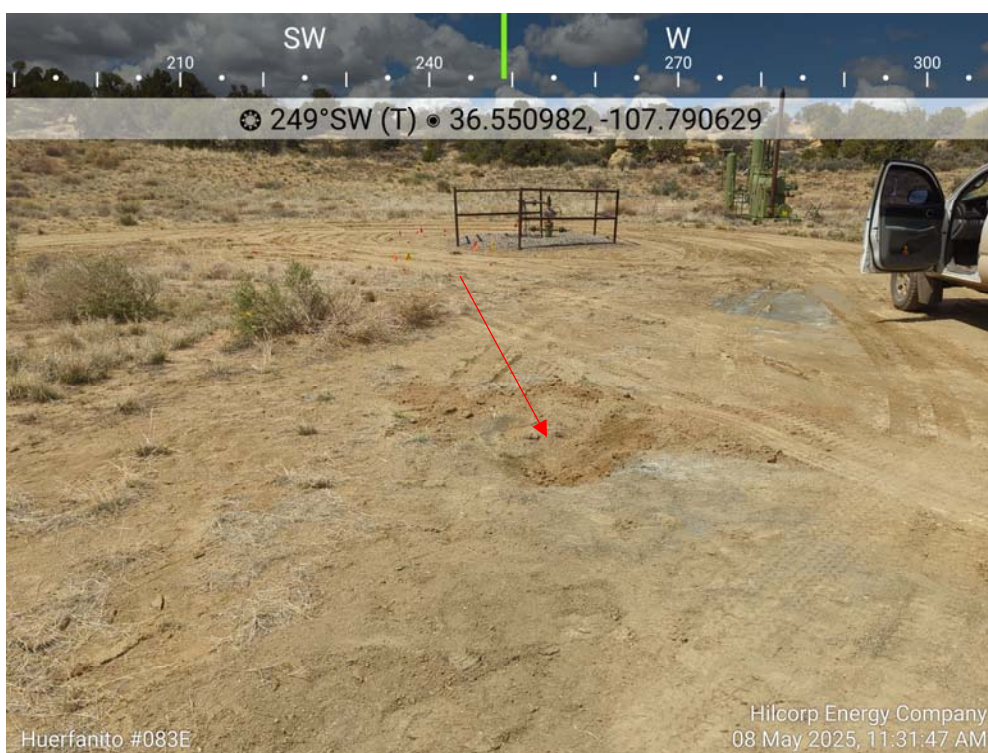
Photo 16: BH-06 (18-20') collected south of bermed area. Bore hole backfilled with grout.
