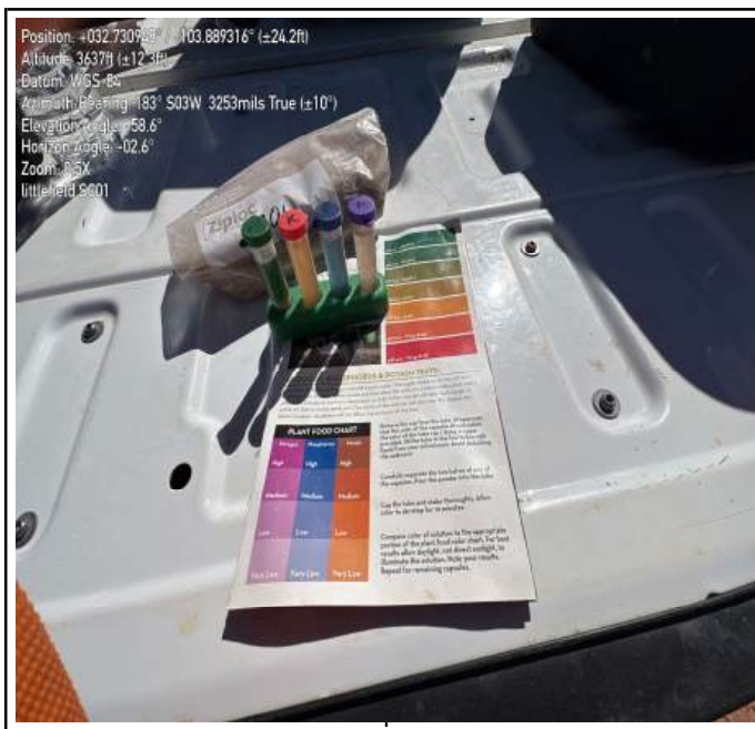
Photograph 8 Date: 02/27/2026 Description: Nutrient testing activities for Soil Cover (SC01).
