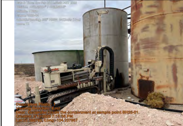
Geoprobe inside the containment at sample point BH26-01.
