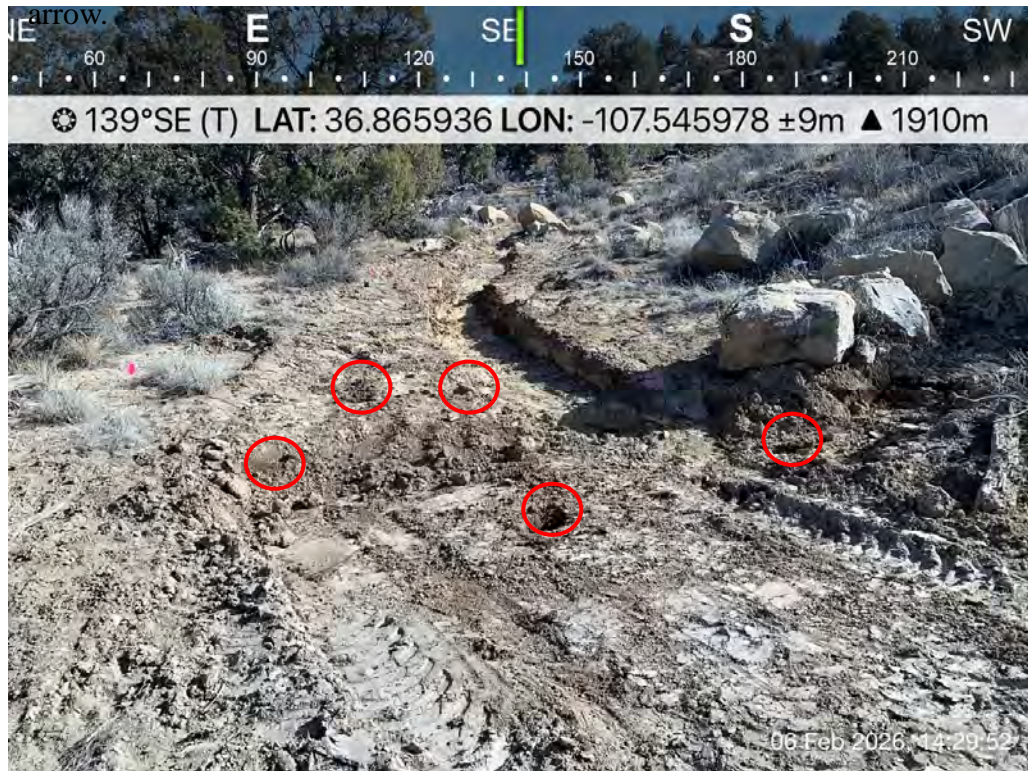
Photo 32: SS31 collected as a 5pct sample from the release area excavation within the drainage.
