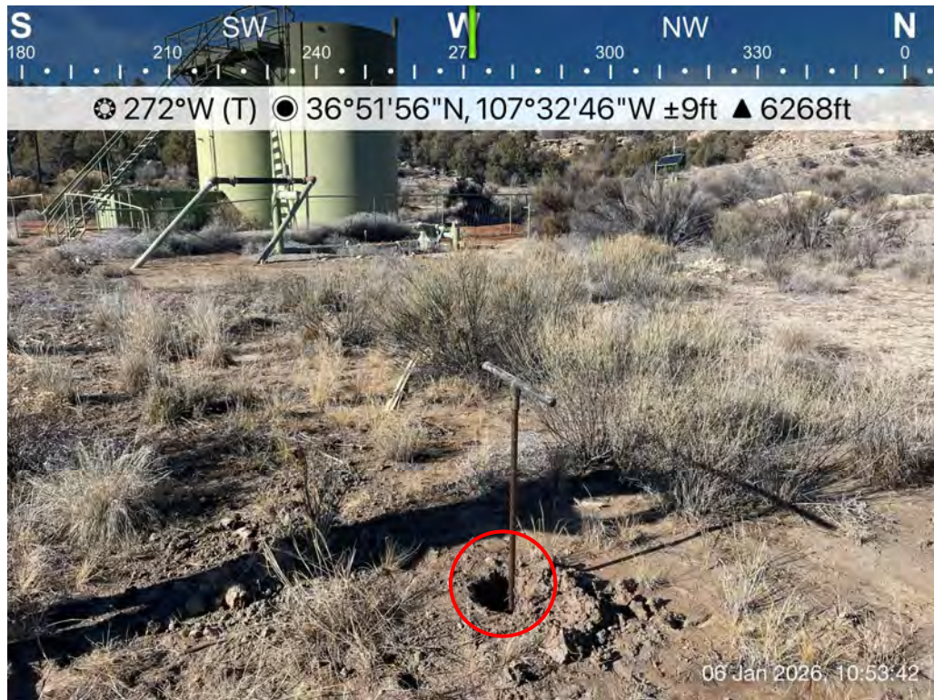
Photo 4: SS03 collected from the same location as SS02 at 30 inches below ground surface.
