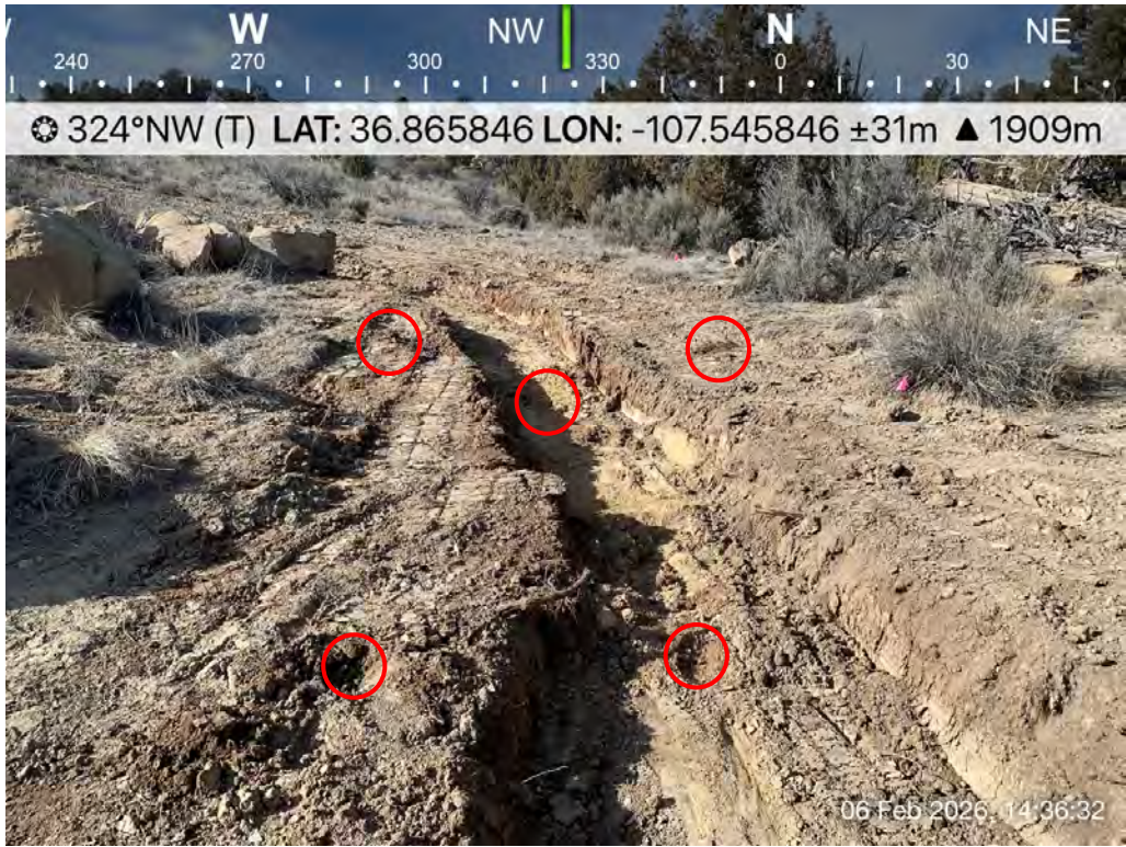
Photo 33: SS32 collected as a 5pct sample from the release area excavation within the drainage.
