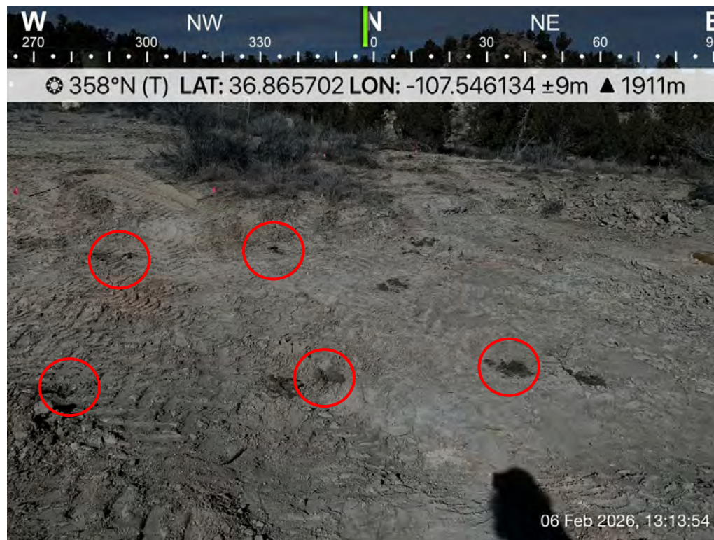
Photo 24: SS23 collected as a 5pct sample from the base of the release area excavation.
