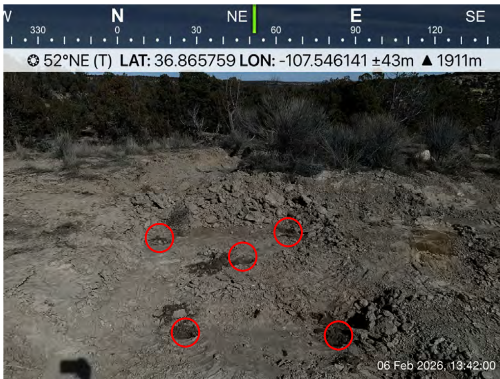
Photo 27: SS26 collected as a 5pct sample from the base of the release area excavation.
