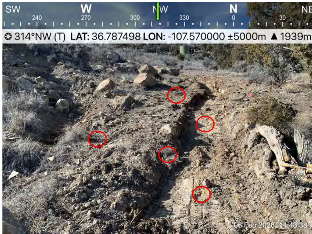
Photo 34: SS33 collected as a 5pct sample from the release area excavation within the drainage.
