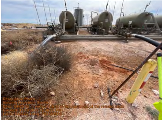
BH25-08, a vertical taken in the northeast of the release stain borehole advanced down to 5ft
