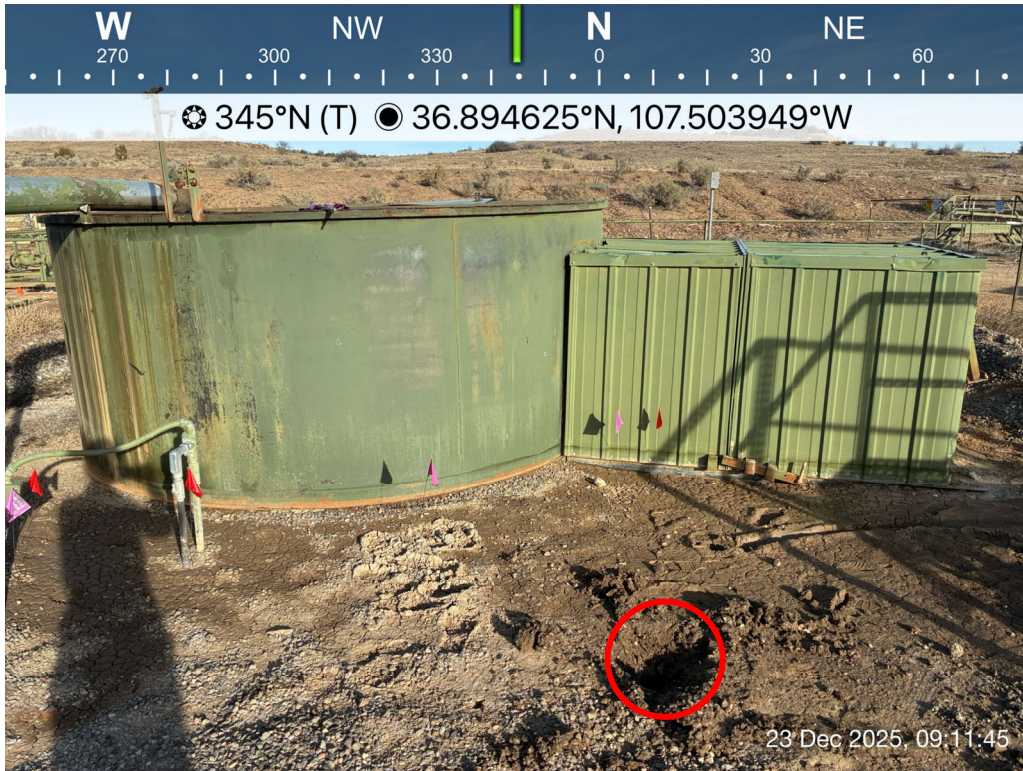
Photo 3: SS01 and SS02 collected from the release area, SS02 collected as a vertical delineation sample three feet below ground surface.
