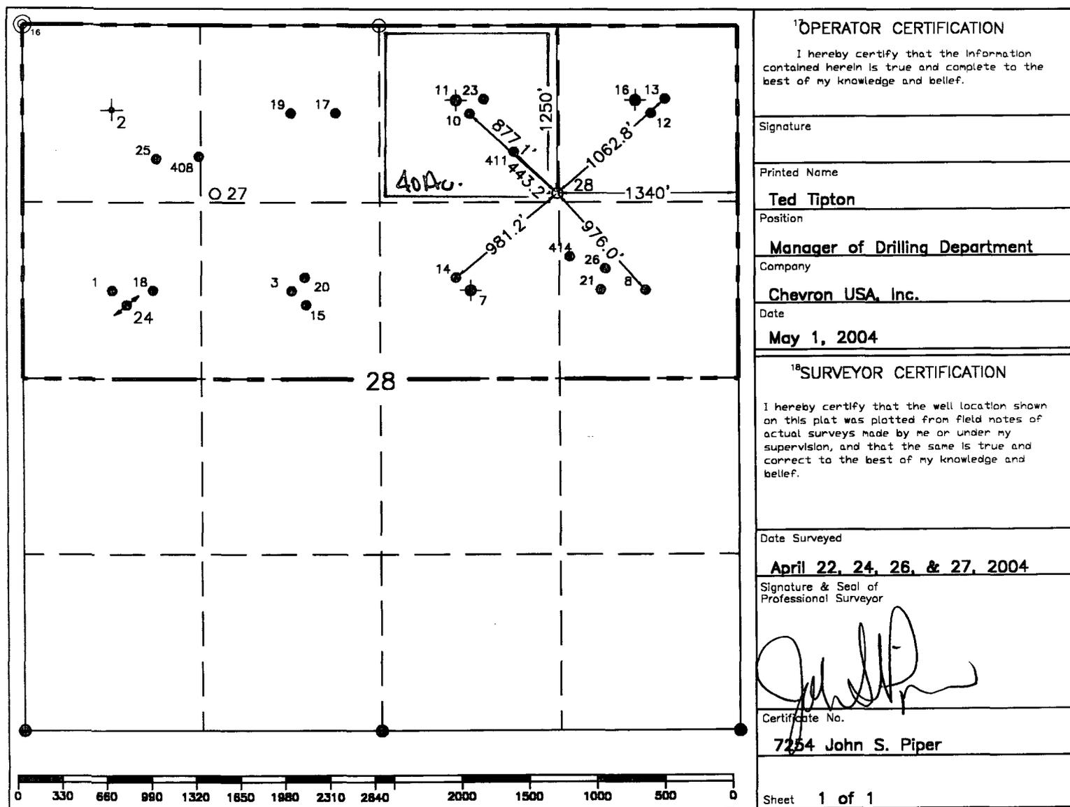
○ = Staked Location ● = Producing Well = Injection Well ◊ = Water Supply Well ⊕ = Plugged & Abandon Well
