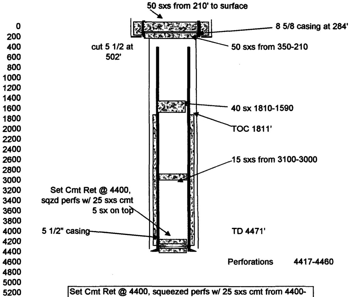
Set Cmt Ret @ 4400, squeezed perfs w/ 25 sxs cmt from 4400-4471, 5 sx on top of retainer. 15sx from 3100-3000, squeezed shot at 1810 w/ 40 sxs cmt to 1590', cut csg at 502', 50 sx 350 to 210', 50 sx 210 to surface
