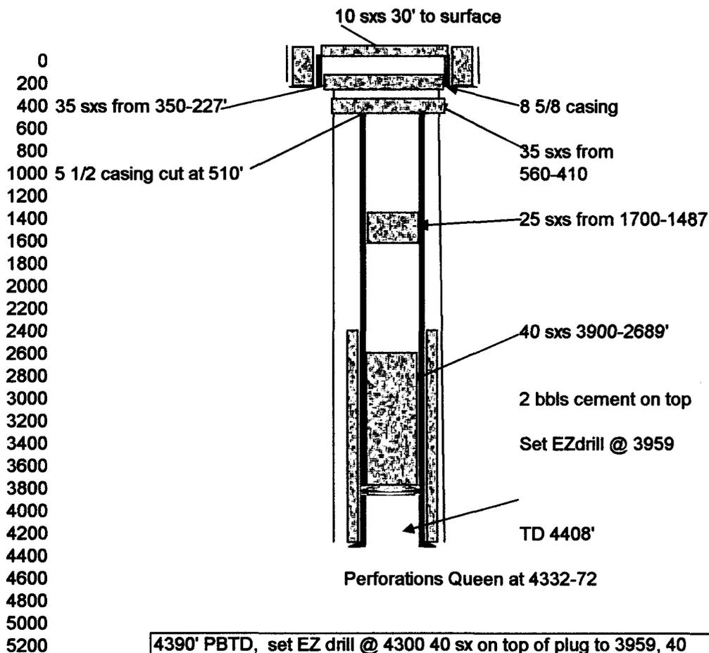
4390' PBD, set EZ drill @ 4300 40 sx on top of plug to 3959, 40 sx from 3900-2689, cut 5 1/2' csg at 510, 25 sx from 1700-1487, 35 sx from 560-410, 35 sx from, 350-227, 10sx from 30 to surface
