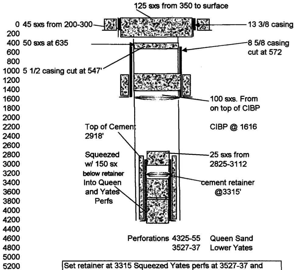
Set retainer at 3315 Squeezed Yates perfs at 3527-37 and Queen at 4325-55 w/ 150 sx. 50sx @ 2825-3112, 50sx from 1500-1712', CIBP@1616 w 50 sx cement on top, 50 sx @ 635, 100sx@350, 25sx @ 30' to surface
