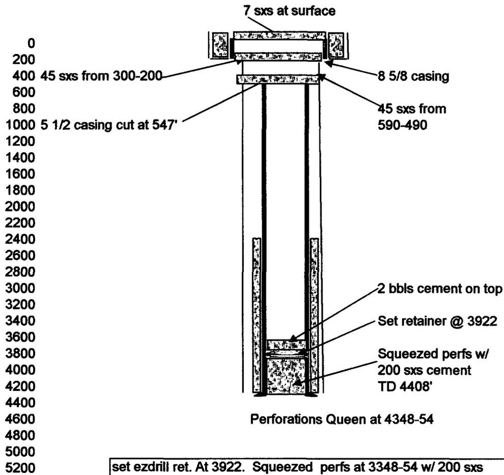
set ezdrill ret. At 3922. Squeezed perms at 3348-54 w/ 200 sxs cement. 2 bbls on retainer. Cut csg at 547. 45 sxs cement 590-490, 45 sxs from 300-200, 7 sxs at surface.
