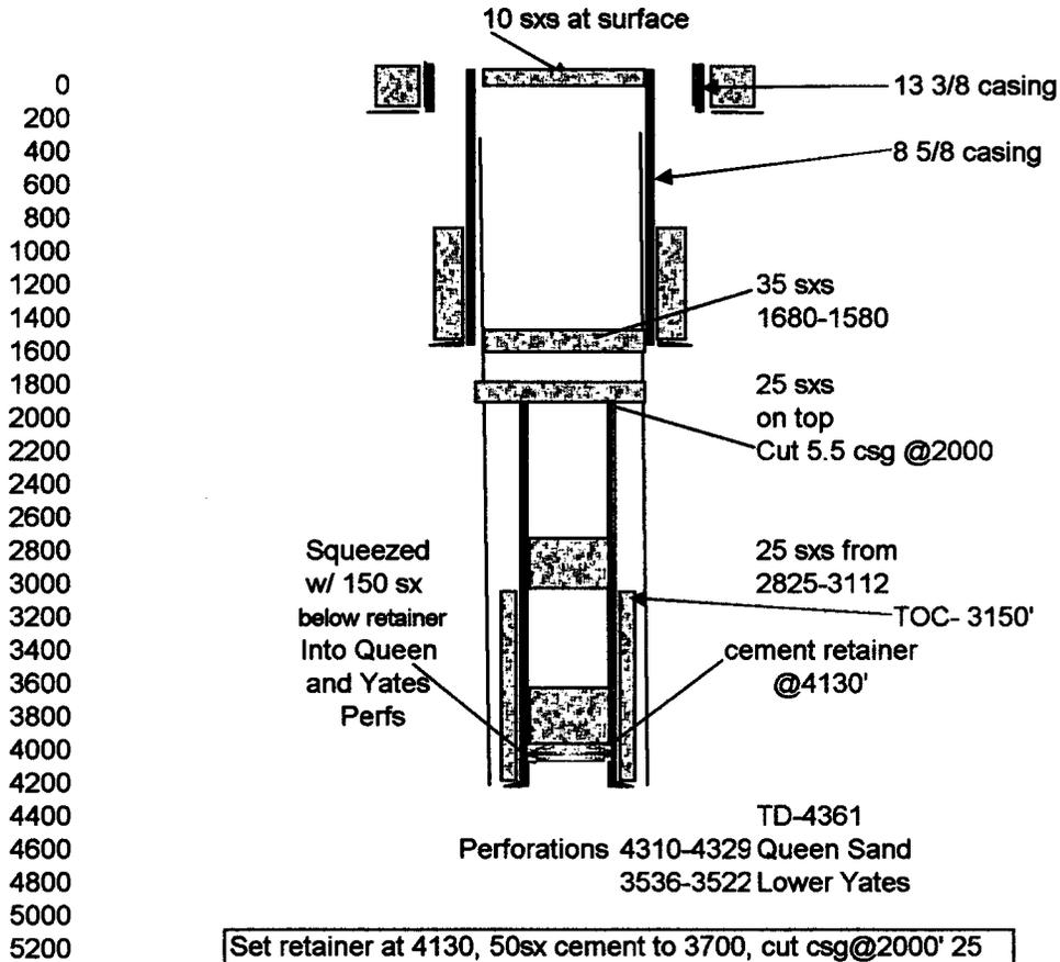
Set retainer at 4130, 50sx cement to 3700, cut csg@2000' 25
