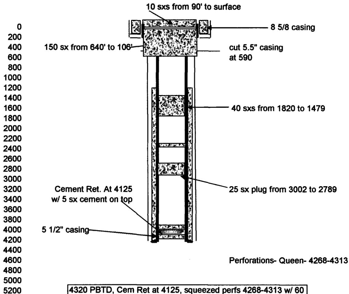
4320 PBTB, Cem Ret at 4125, squeezed perms 4268-4313 w/ 60 sxs. 5 sxs on Ret. 25 sx plug from 3002 to 2789, 40 sxs from 1820 to 1479, cut 5 1/2 at 590' 150 sxs to 190', 10 sx from 90' to surface.
