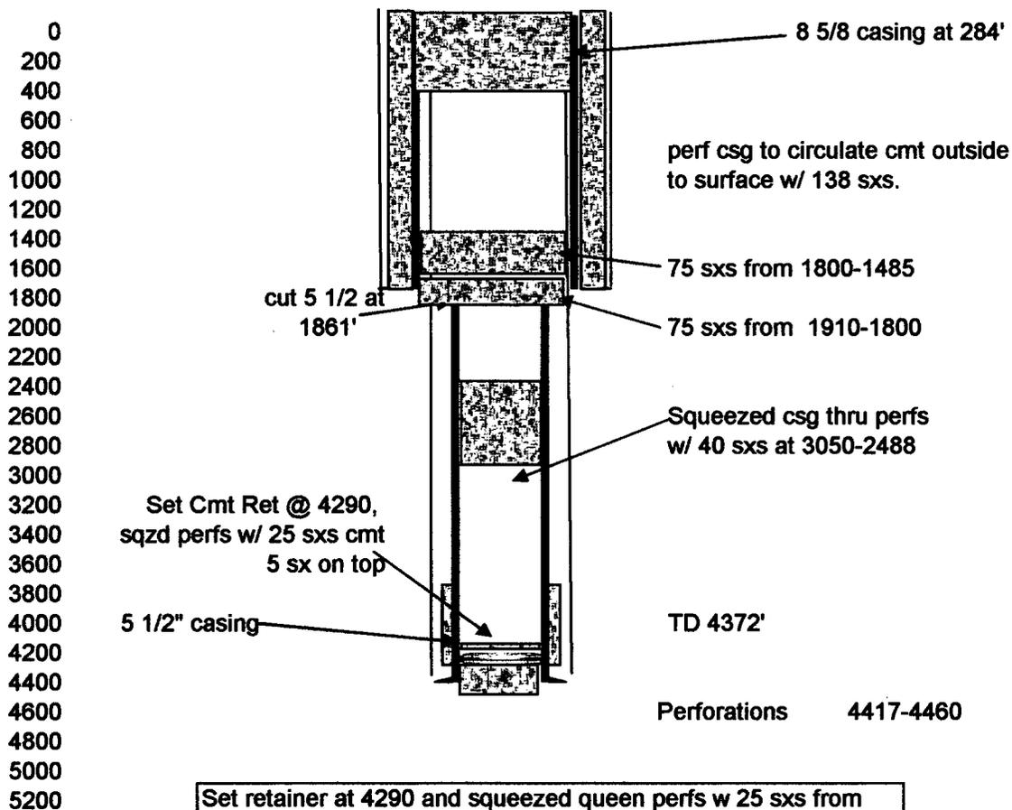
Set retainer at 4290 and squeezed queen perfs w 25 sxs from 4417-4460 w/ 5 sx on top to 4240. Squeezed casing leak thru perfs at 3050 to 2488 w 40 sxs. Cut csg at 1861', 75 sxs from 1910-1800, 75 sxs from 1800-1485, perforated casing at 500 and 200' to circulate outside casing w 138 sxs. add 130 sx cmt to surface.
