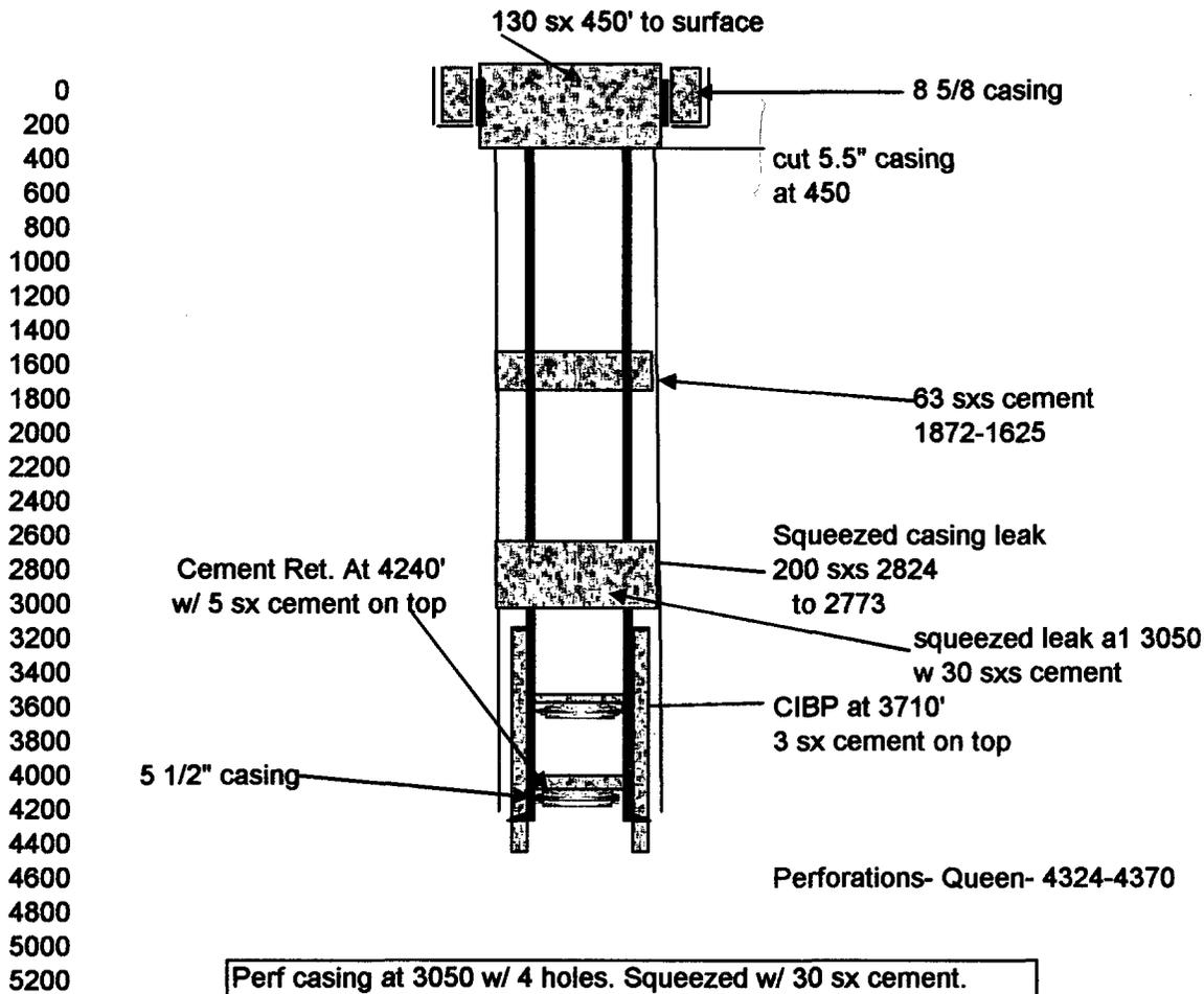
Perf casing at 3050 w/ 4 holes. Squeezed w/ 30 sx cement.
