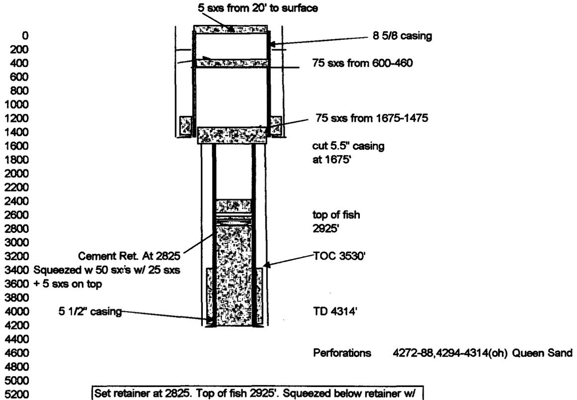
Set retainer at 2825. Top of fish 2925'. Squeezed below retainer w/ 50 sxs of cement w/ 5 sx on top. TOC 2785 . 30 sxs from 2750-2500 . Cut casing at 1675. 75 sx from 1675 to 1475. 75 sxs from 600-460. 5 sxs from 20' to surface
