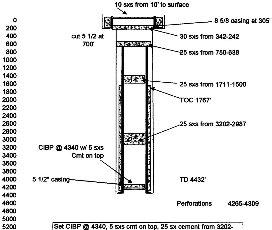
Set CIBP @ 4340, 5 sxs cmt on top, 25 sx cement from 3202-2987, 25 sx from 1711-1500, cut 5 1/2 csg at 700', 25 sx cmt from 750-638, 30 sx from 342-242, 10 sx from 10' to surface.
