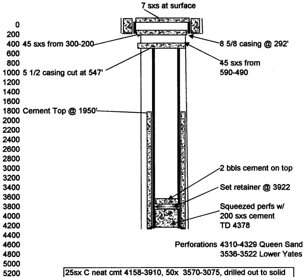
25sx C neat cmt 4158-3910, 50x 3570-3075, drilled out to solid cmt at 4127, CIBP @ 3915 95sx to 3000, cut csg at 1775. 5x 1620-1890, 50x 400-200, 20x 120 to surface
