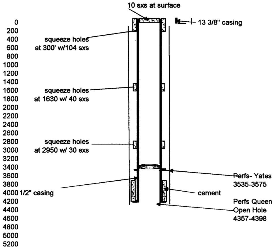
CIBP @ 3505 w/ 5 sxs on plug, 4 squeeze holes @ 2950. Squeeze w/ 30 sxs Pwef 4 squeeze holes @ 1630, Squeeze w/ 40 sxs. Perf 4 squeeze holes @ 300'. Circulate 104 sxs 10 sxs @ surface
