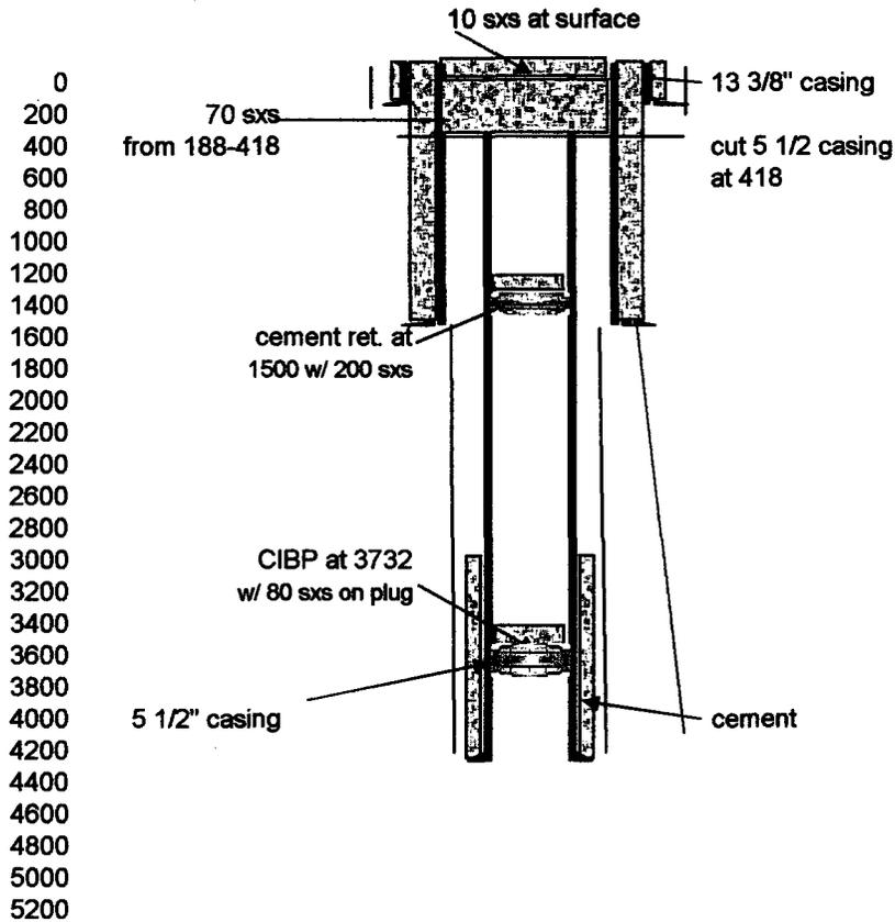
CIBP @ 3732 w/ 80 sxs on plug. Cmt retainer @ 1500 squeezed w/200 sxs . Cut 5 1/2 @ 418 70 sxs 188 - 418 10 sxs @ surface
