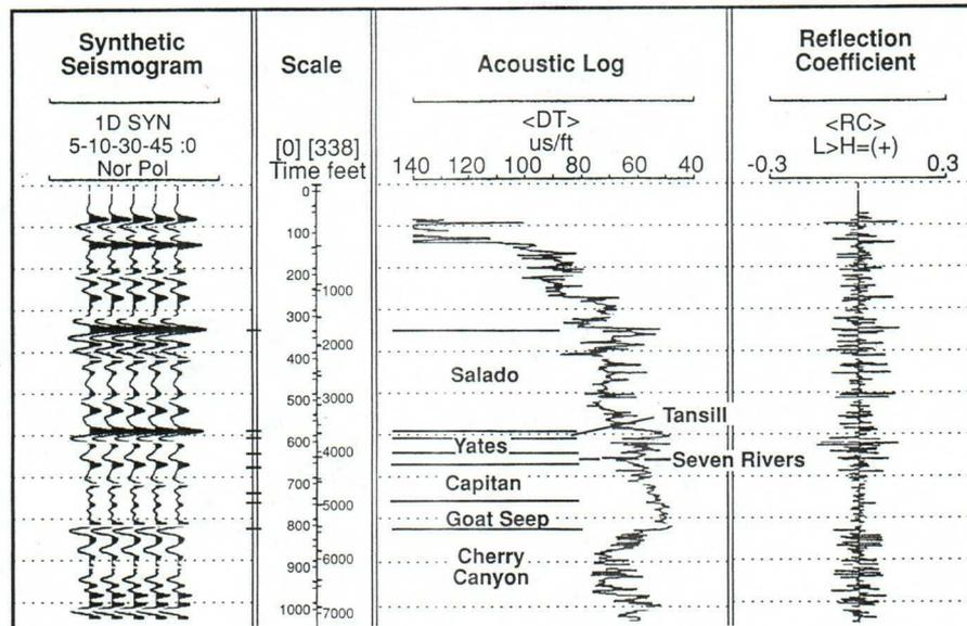
FIG. 5.—Synthetic seismogram for Humble Oil and Refining (Exxon) Davidson-Federal No. 1 well showing the relationship between acoustic log, seismic reflections, and stratigraphy of the Capitan depositional system.
