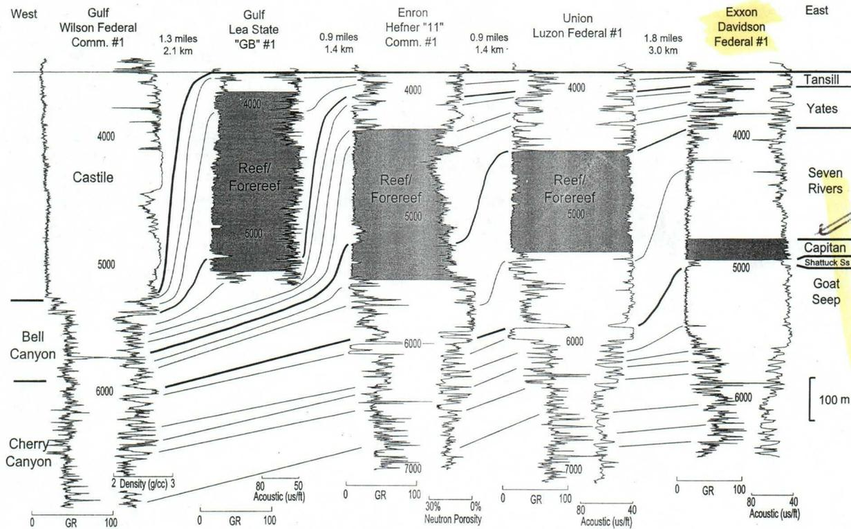
FIG. 6.—Wireline log cross-section using wells located near the seismic line shown in Figs. 3 and 4. Stratigraphy and shelf-to-basin correlations for the Capitan depositional system are shown. Section is approximately dip-oriented. Correlations follow seismic geometries as well as log patterns. Section is stratigraphic; datum is top Tansill Formation except for basin well where top Castile is used. Well locations are shown in Fig. 1.
