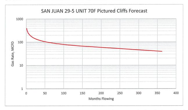
The forecast for Pictured Cliffs production has been generated using a typical well production profile of PC gas production in the surrounding production trend.
