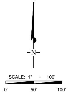
ALL BEARINGS, DISTANCES, AND COORDINATE VALUES CONTAINED HEREON ARE GRID BASED UPON THE NEW MEXICO COORDINATE SYSTEM, EAST ZONE OF THE NORTH AMERICAN DATUM 1983, U.S. SURVEY FEET
