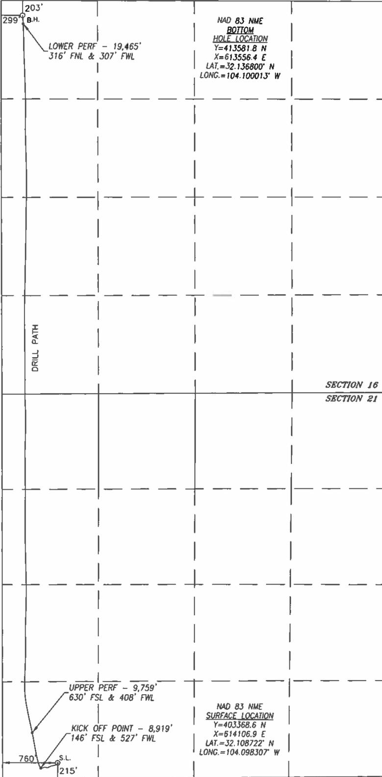
SURFACE INFO AND BOREPATH SHOWN HEREON IS BASED ON DIRECTIONAL SURVEY REPORT PROVIDED BY COG OPERATING, LLC FOR THE MYOX 21 STATE COM #31H SUPPLIED TO HARCROW SURVEYING, LLC ON NOVEMBER 7, 2019
