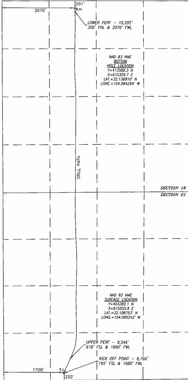
SURFACE INFO AND BOREPATH SHOWN HEREON IS BASED ON DIRECTIONAL SURVEY REPORT PROVIDED BY COG OPERATING, LLC FOR THE MYOX 21 STATE COM #34H SUPPLIED TO HARCROW SURVEYING, LLC ON NOVEMBER 14, 2019
