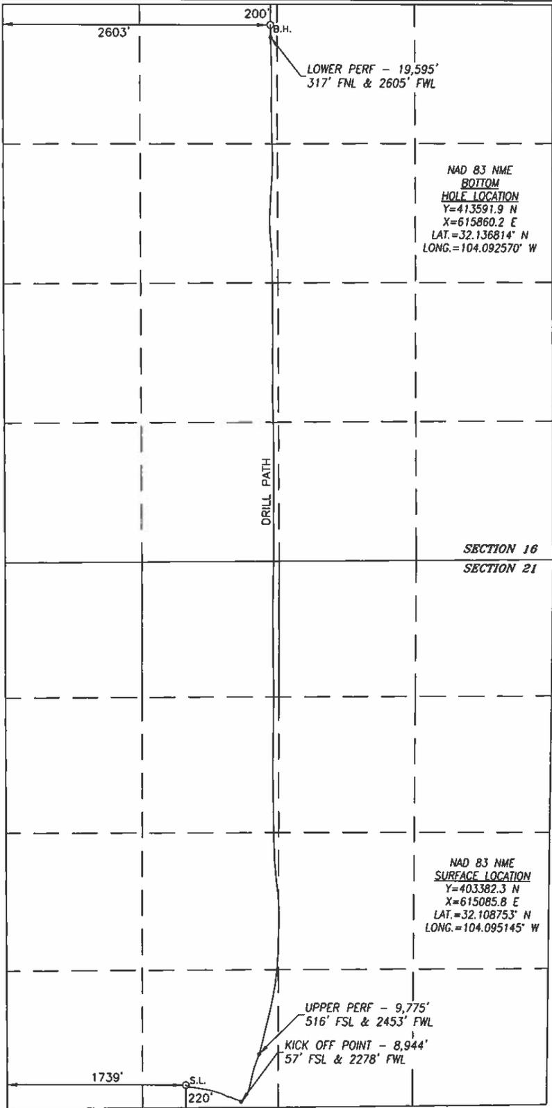
SURFACE INFO AND BOREPATH SHOWN HEREON IS BASED ON DIRECTIONAL SURVEY REPORT PROVIDED BY COG OPERATING, LLC FOR THE MYOX 21 STATE COM #35H SUPPLIED TO HARCROW SURVEYING, LLC ON NOVEMBER 14, 2019
