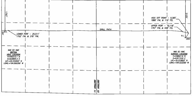
SURFACE INFO AND BOREPATH SHOWN HEREON IS BASED ON DIRECTIONAL SURVEY REPORT PROVIDED BY COG OPERATING, LLC FOR THE HOWITZER FEDERAL COM #805H SUPPLIED TO HARCROW SURVEYING, LLC ON JANUARY 20, 2020
