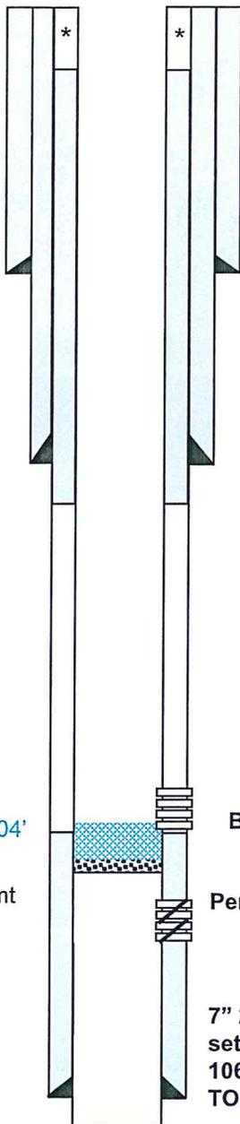
\* 7" csg repair @ 472' pulled and re-installed 7" w/ csg bowl and lead seal 1974
