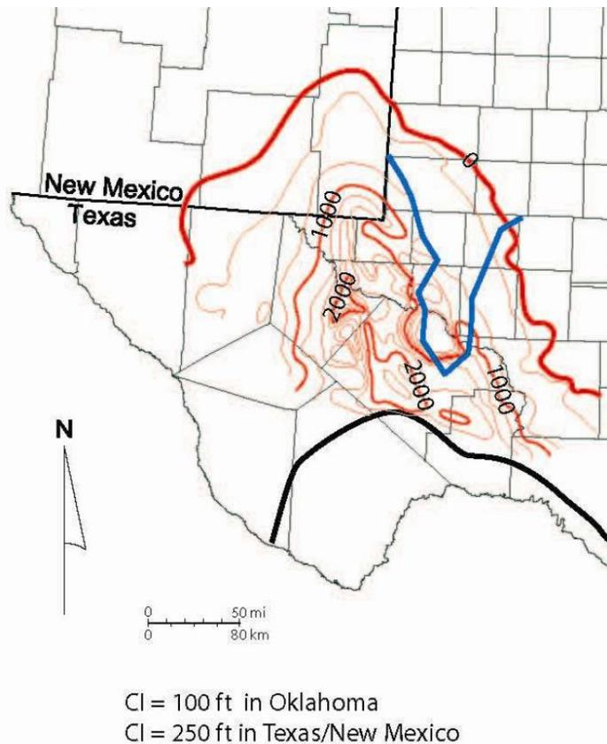
Data from the Amoco Federal CW Com 1 (30-025-28119) show that the thickness of the Simpson in the Antelope Ridge area of Lea County (Section 3 24S 34E) is about 450 feet thick with. This is consistent with Figure 4 of the BEG paper (probably because this well was used to produce the isopach map).
