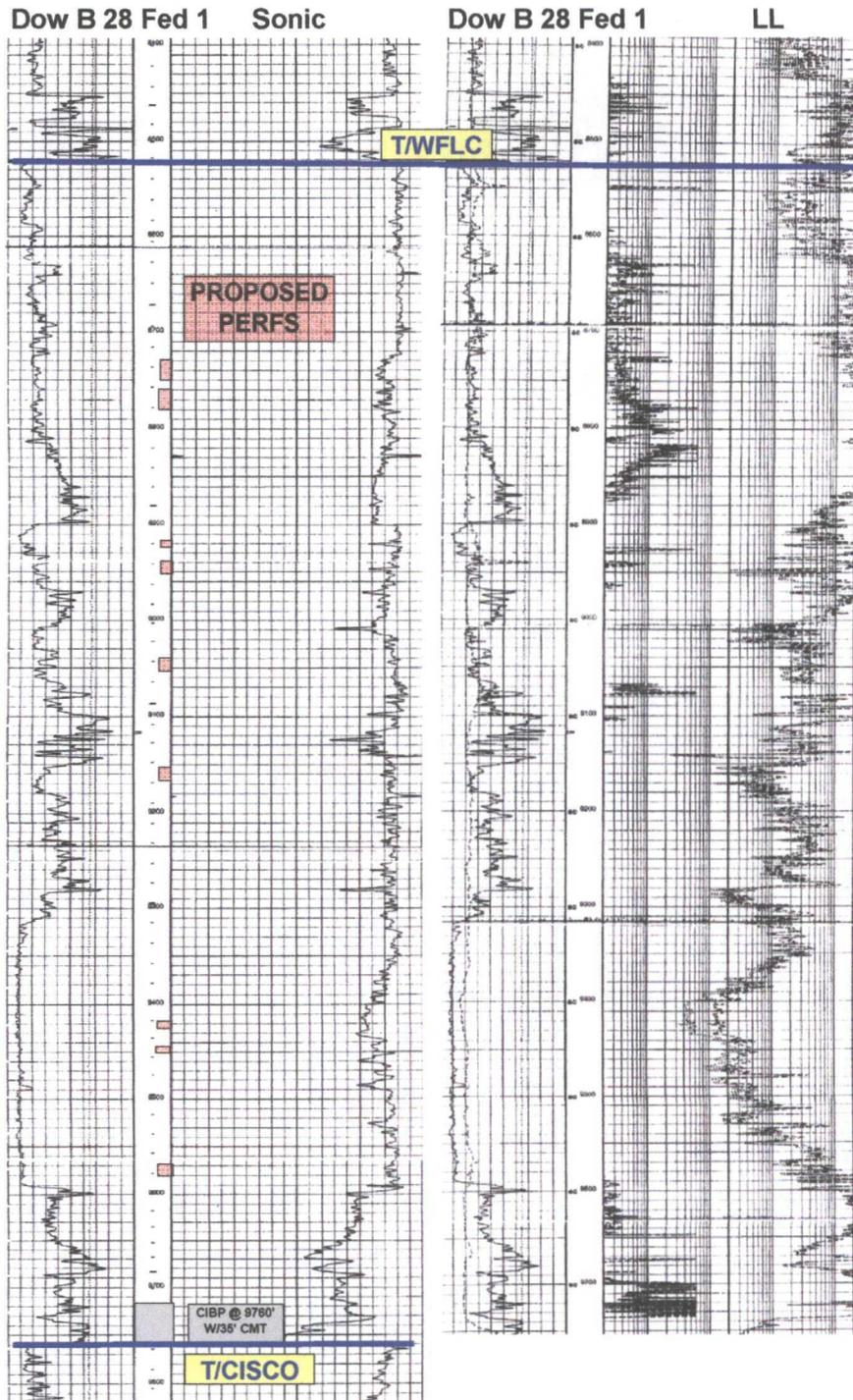
Figure 7: Dow "B" 28 No 1 Borehole Sonic and Duel Lateral Logs
