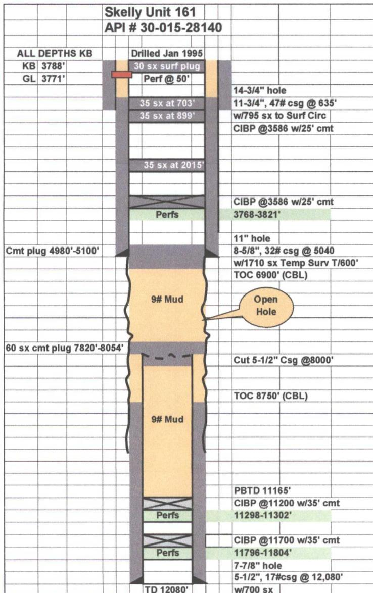
**Figure 10: Current Wellbore Schematic Skelly Unit Well 161**
