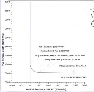
Azimuths to Grid North True North: -0.13° Magnetic North: 7.64°
