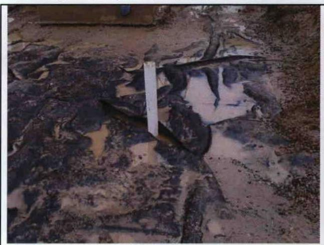
6.) View of sample location CS-3 in pooling area. PVC used to keep water out of boring. Water on liner drained to ground from above, after liner was cut for sample access.
