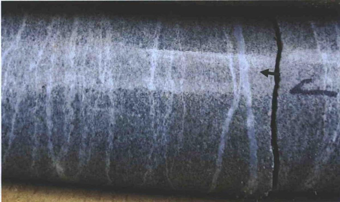
**Photo 11:** Gray fine to medium, arkosic SANDSTONE, with fibrous gypsum vein deposits (608 to 610 feet).
