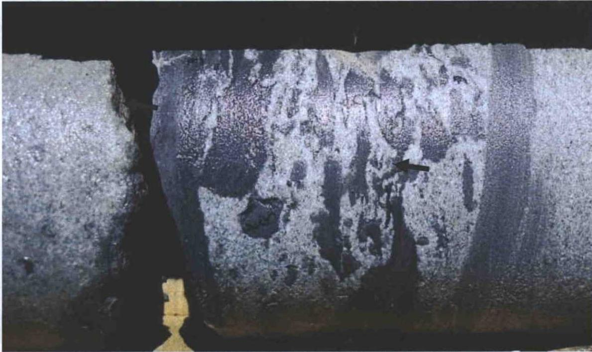
**Photo 5:** Gray fine to medium SANDSTONE with rip-up mud clasts (128 to 130 feet).
