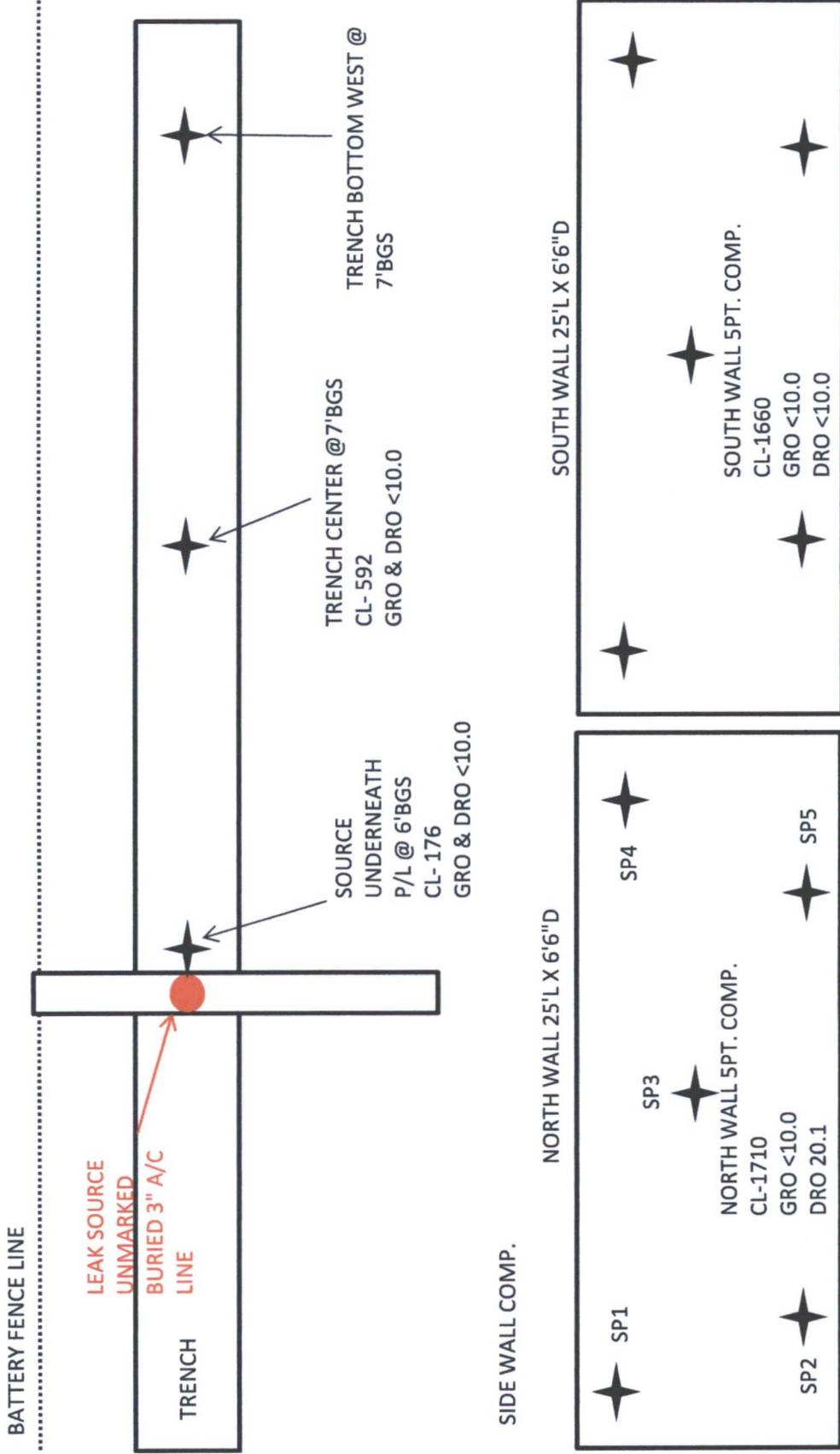
TARGA / RHOMBUS BATTERY LEAK
