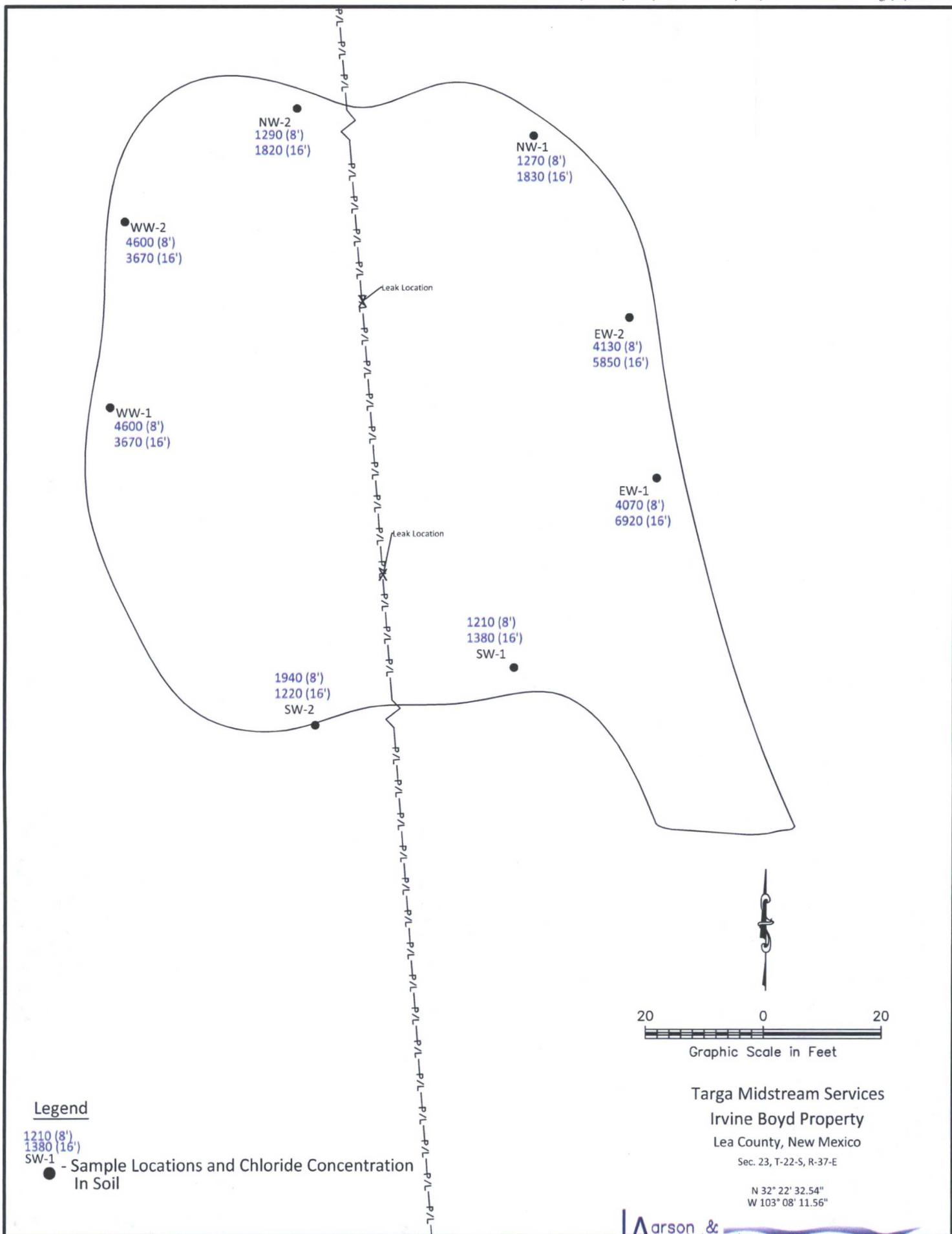
Figure 4 - Chloride Concentration in Soil
