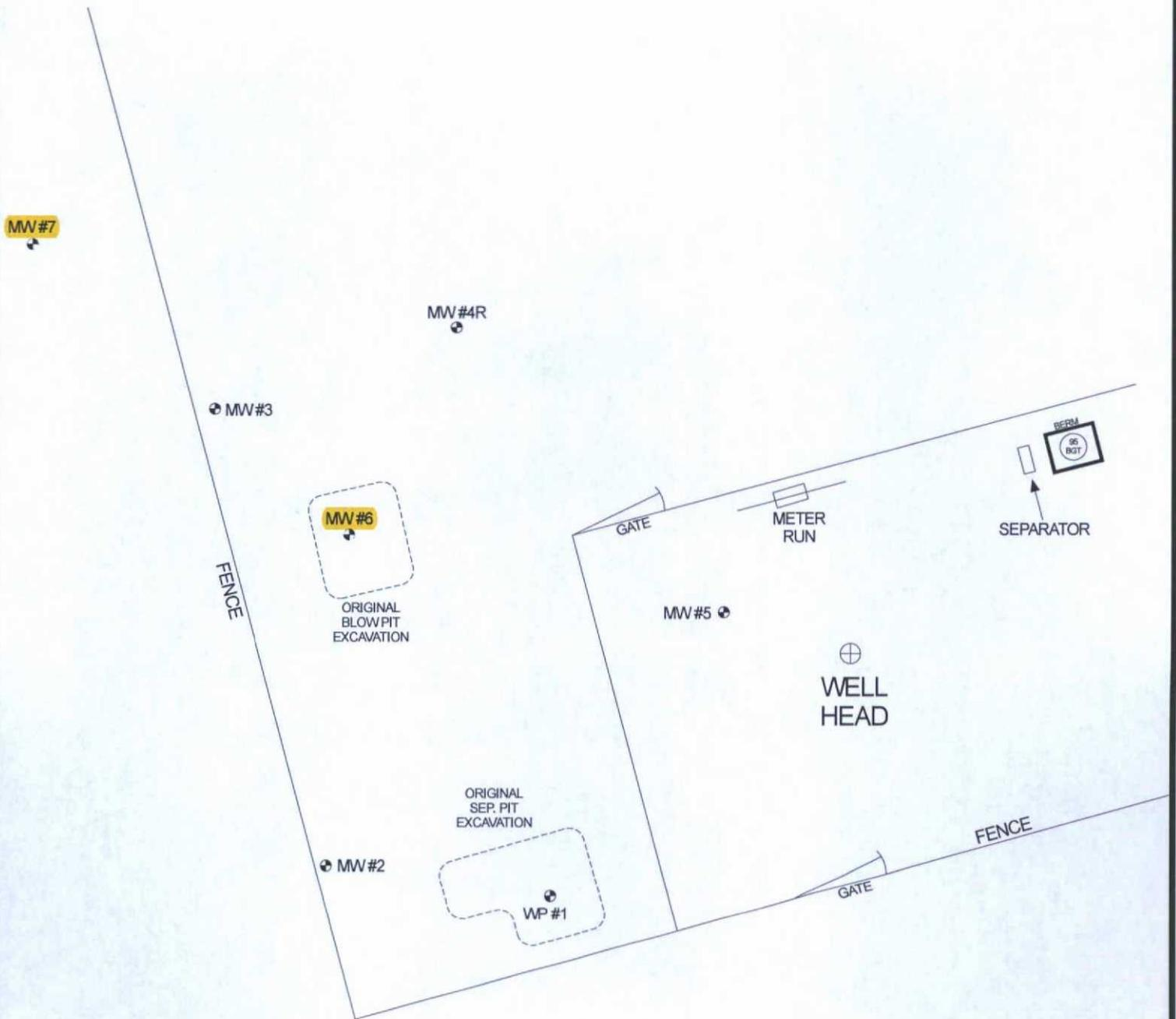
MONITOR WELL LOCATIONS ARE ONLY AS ACCURATE AS THE INSTRUMENTS USED IN OBTAINING THE FOOTAGE AND BEARING FROM THE WELL HEAD (BRUNTON COMPASS AND LASER RANGE FINDER). ALL OTHER STRUCTURES DISPLAYED ON THE SITE MAP ARE SOLELY FOR REFERENCE AND MAY NOT BE TO SCALE.
