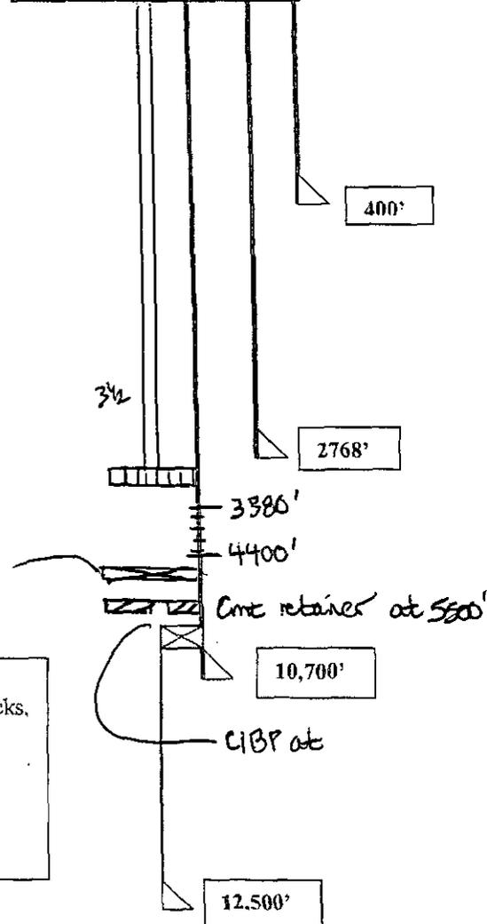
4.5" 13.5# P110 liner, 6.15" hole, cemented to top of liner w/ 295 sacks, circulated 55 sacks off of liner top. Top of liner is 10,277'
