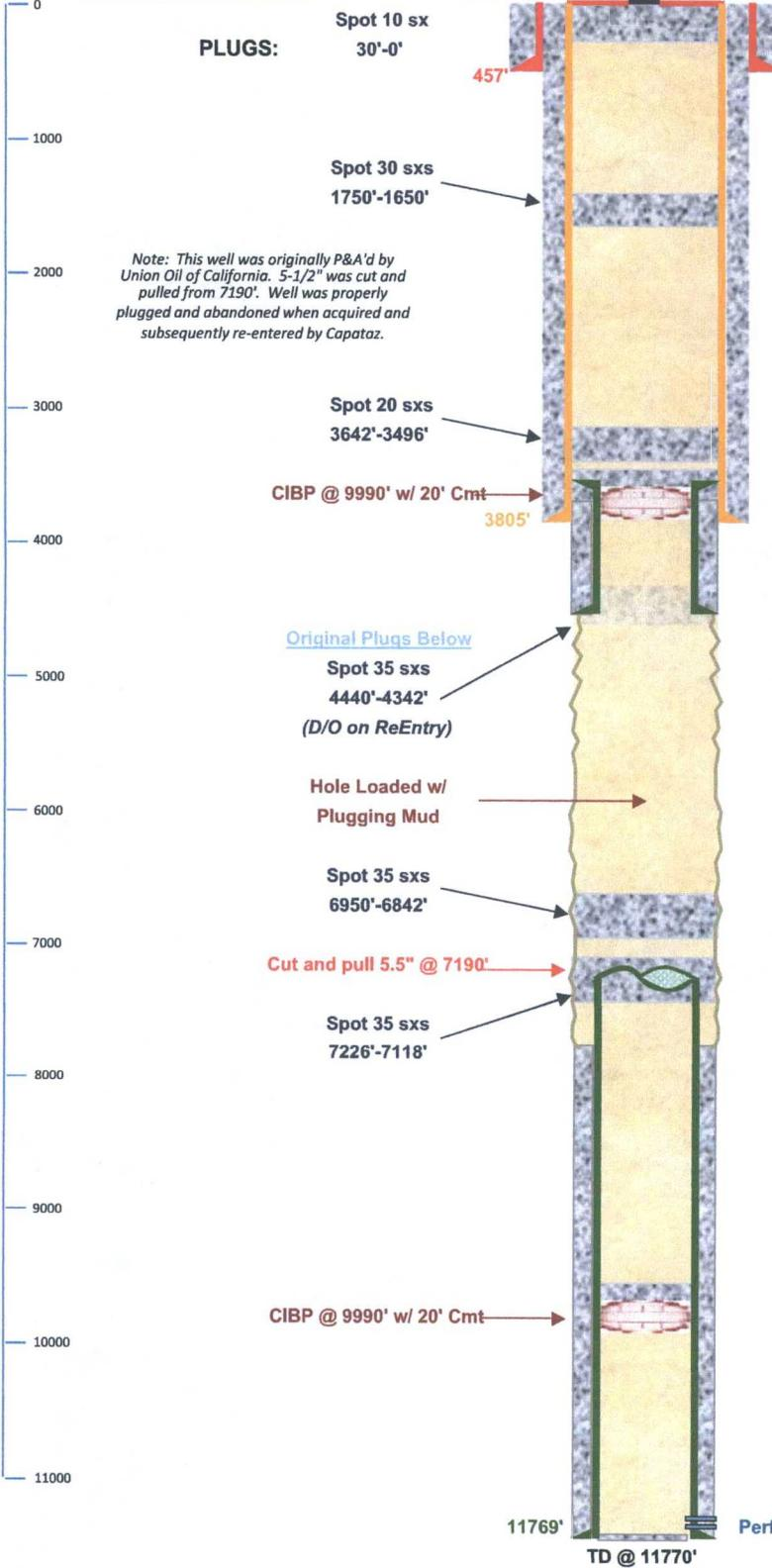
Note: This well was originally P&A'd by Union Oil of California. 5-1/2" was cut and pulled from 7190'. Well was properly plugged and abandoned when acquired and subsequently re-entered by Capataz.
