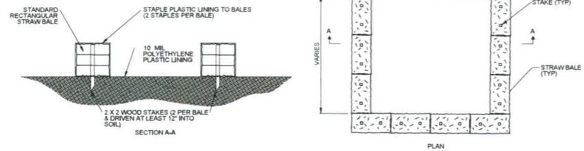
CONCRETE TRUCK WASH OUT FACILITY (CTW) N.T.S.
