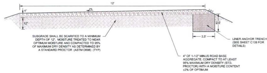
**PRODUCED WATER PIT ACCESS ROAD SECTION** 1
