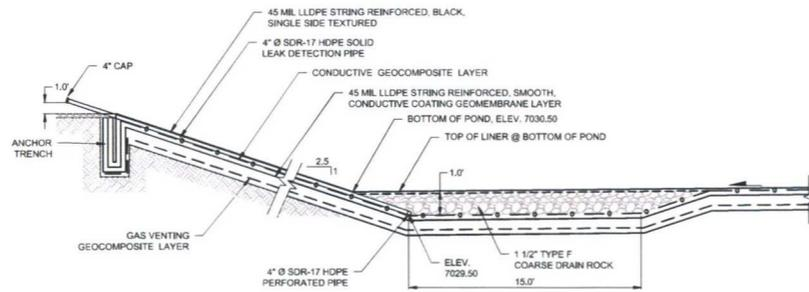
**PRODUCED WATER PIT LEAK DETECTION** 3
