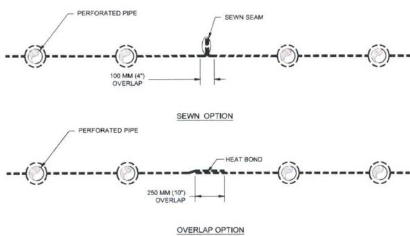
**GAS VENTING GEOCOMPOSITE PANEL JOINING OPTIONS FOR SIDE**
