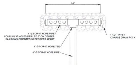
**LEAK DETECTION SYSTEM PIPE DETAIL** 4
