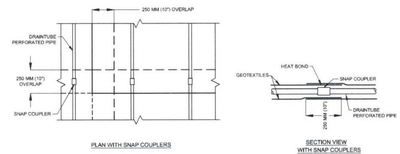
**GAS VENTING GEOCOMPOSITE PANEL JOINING OPTIONS FOR END**
