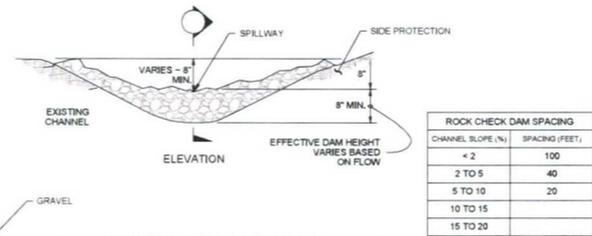
EXTENDED SECTION (A) ROCK CHECK DAM (RD) N.T.S.
