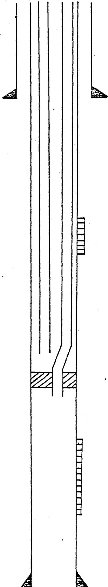
8-5/8", 24#, K-55 casing set at 240', cemented with 160 sacks cement.
