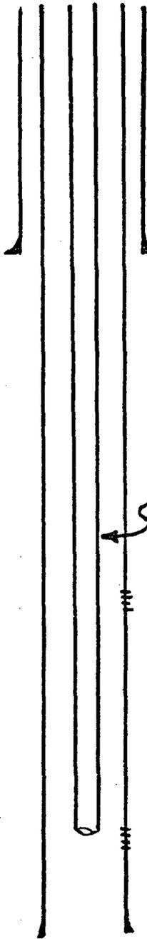
8-5/8" OD Casing set at 120' and cemented to surface
