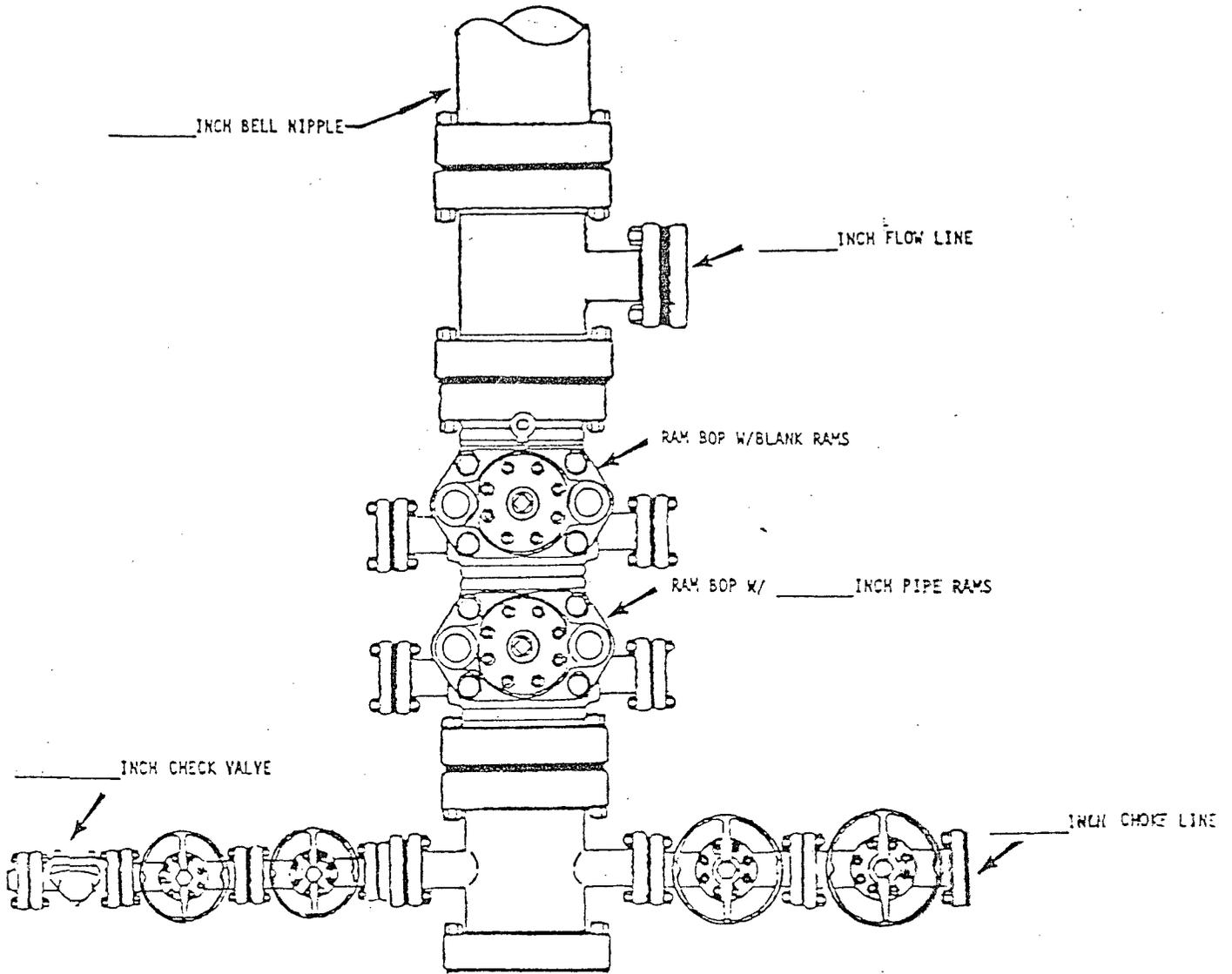
\*NOTE: ALL VALVES ARE METAL-TO-METAL SEAL AND FLANGED. ALL COMPONENTS MUST MEET ABOVE MINIMUM PRESSURE RATINGS. ALL COMPONENTS TO BE TESTED TO RATED PRESSURE AFTER ASSEMBLY AND BEFORE FURTHER DOWNHOLE OPERATIONS MAY BE CONDUCTED.
