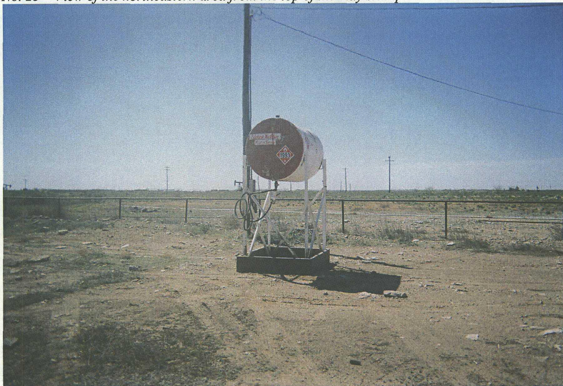
No. 24 – View of a diesel fuel container brought onsite for equipment refueling with a secondary containment vessel.
