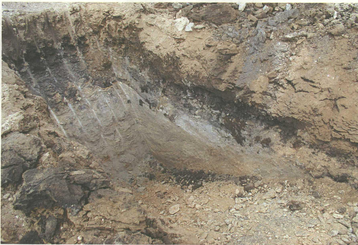
No. 45 – View of the subsurface within test pit TP-2 located near monitoring well MW-2 (petroleum staining to 8 foot depth at this location).
