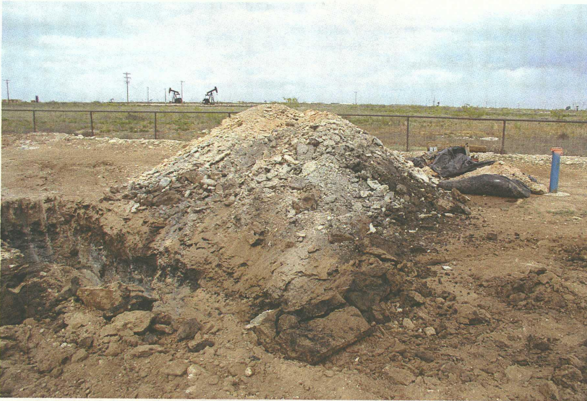
No. 47 – View of stained soil material from test pit (TP-2). The test pit was backfilled with clean soil.
