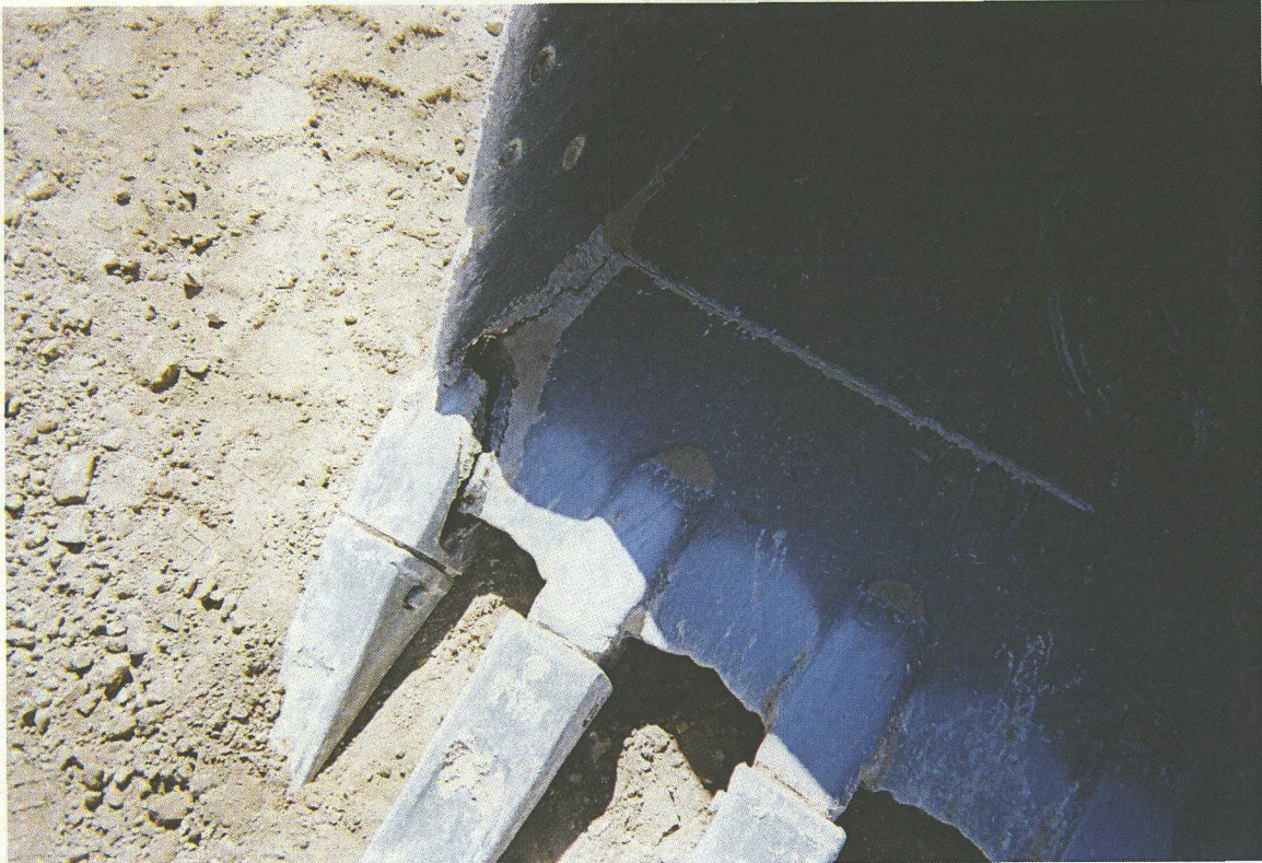
No. 25 – View of broken a tooth of the excavator while excavating around the hard rock areas.
