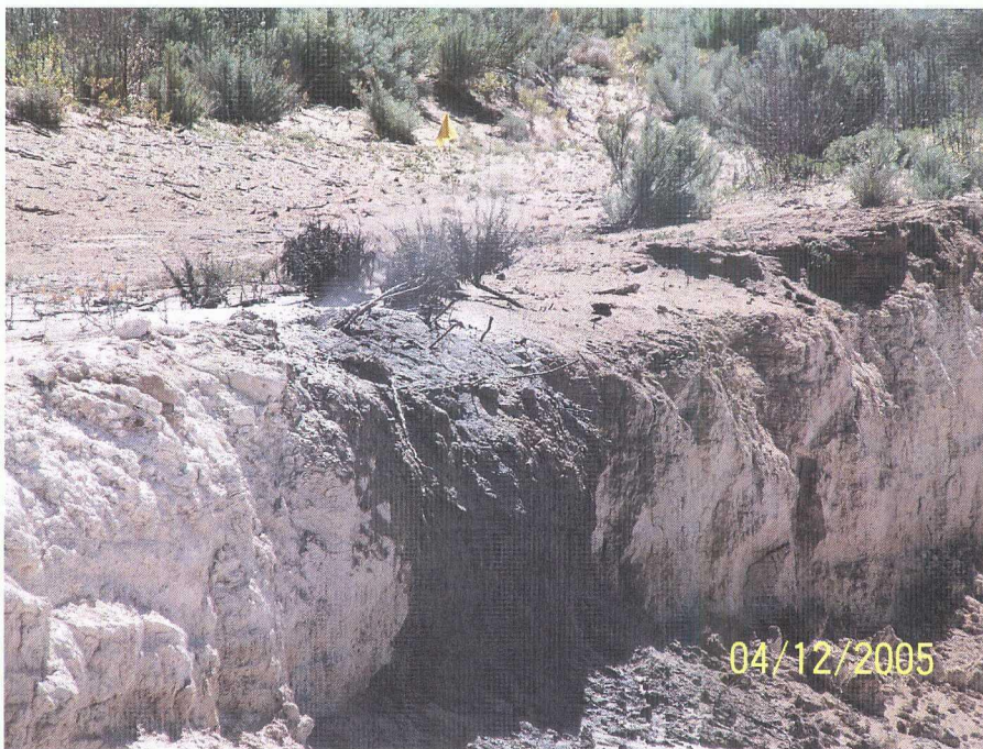
Photograph #8- Looking westerly at natural gas and natural gas liquids release from Sid Richardson pipeline.
