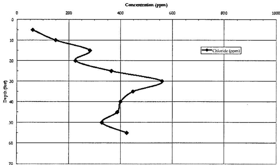
Figure 2: Chloride Concentration vs. Depth for B-32 Boot Site
