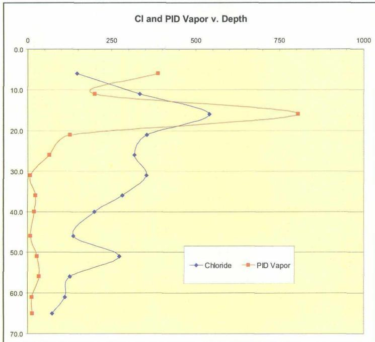
Chloride concentrations reach approximate background levels at a depth of 56 feet bgs. Field evidence demonstrates that the chloride mass resides in the upper two-thirds of the vadose zone.
