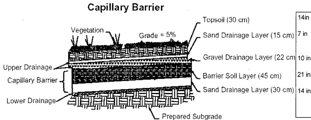
Figure 1: ET Soil Cover Design from SNL Report SAND 2000-2427. Dimensions in inches shown as a modification to the SNL figure.
