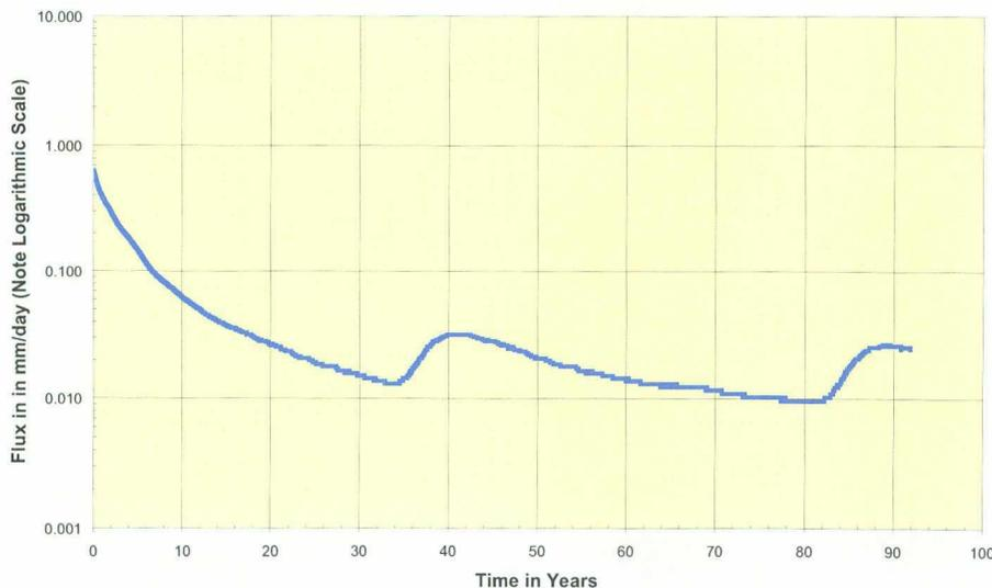
Figures 5 show the results of this simulation experiment. The ET Barrier is installed at time = 1.1 years, representing the present in Figure 4. The HYDRUS-1D simulation of the ET Barrier slows the migration of the vadose zone chloride mass such that ground water may exceed standards for a period of nearly 17 years in the absence of any chloride removal from the aquifer due to pumping.
