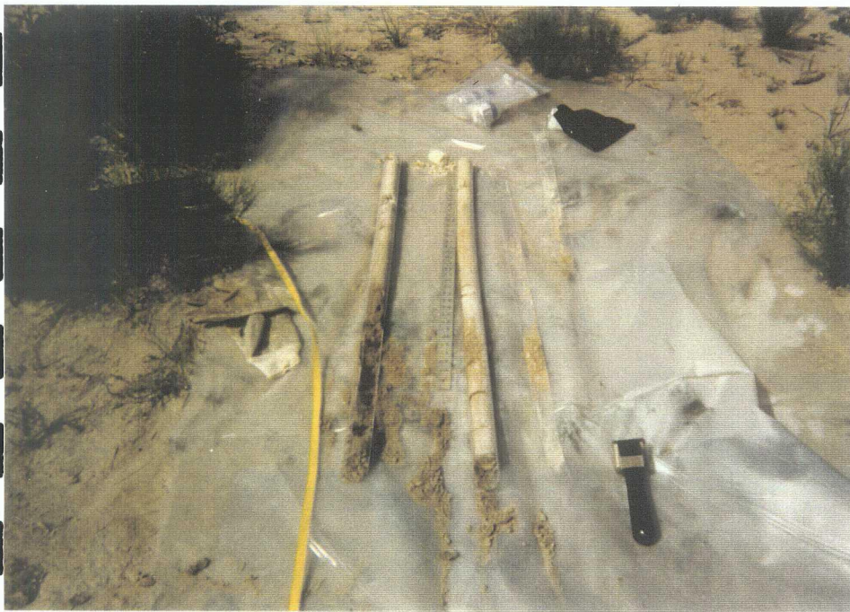
PHOTO 7: Cores 1 and 2 from well #1 showing brown sand at surface overlaying caliche zone. Top of cores are at the bottom of the photo.
