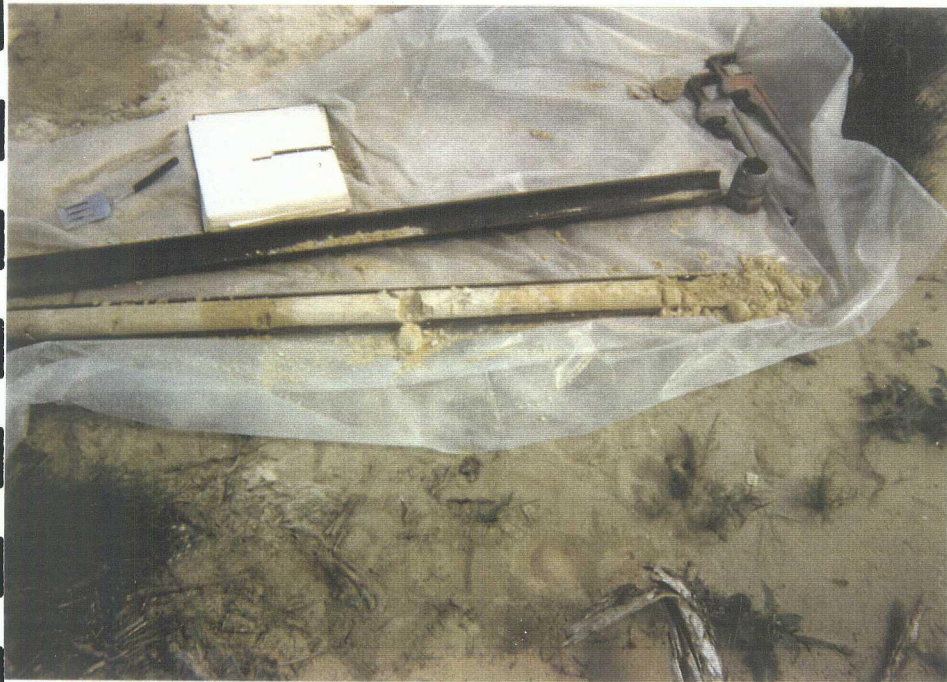
PHOTO 8: Core 2 from well #3 shows hard lime with broken lime section at approximately 10 feet. Top of core is to the left.
