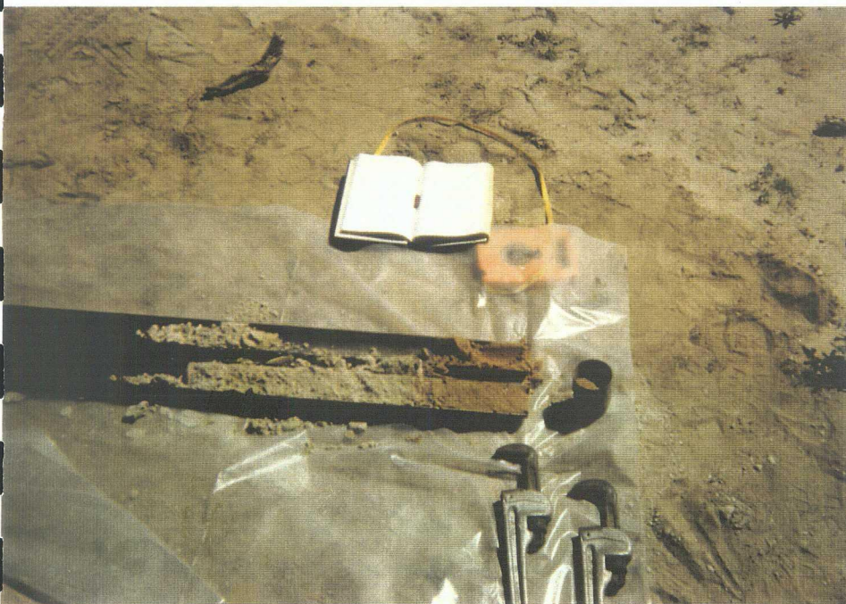
PHOTO 9: Core 5 from well #5 shows red sand at bottom of lime section. Top of core is to the left.
