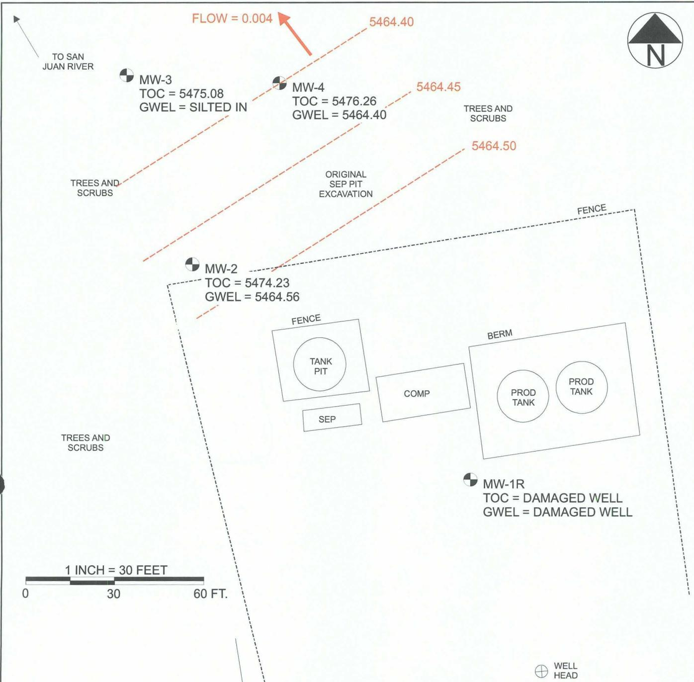
TOC = TOP OF CASING ELEVATION
