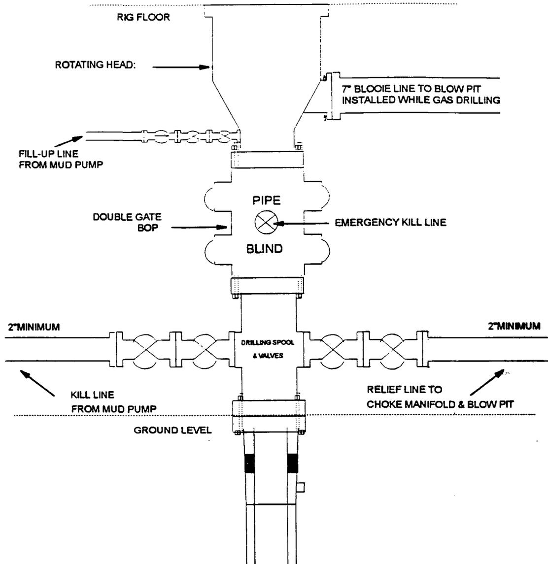
13 5/8" and 11" Bore, 2000psi minimum working pressure double gate BOP to be equipped with blind and pipe rams. A Schaffer Type 50 or equivalent rotating head to be installed on the top of the BOP. All equipment is 2000psi working pressure/ or greater.
