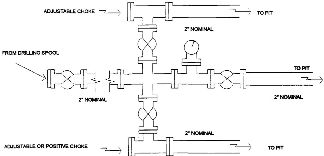
Minimum choke manifold installation from surface to Total Depth.
