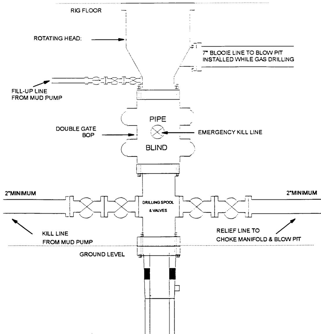
11" Bore, 2000psi minimum working pressure double gate BOP to be equipped with blind and pipe rams. A Schaffer Type 50 or equivalent rotating head to be installed on the top of the BOP. All equipment is 2000psi working pressure/or greater.
