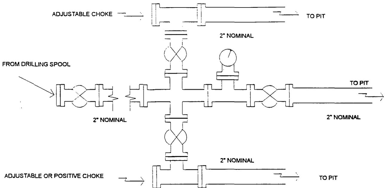
Minimum choke manifold installation from surface to Total Depth.
