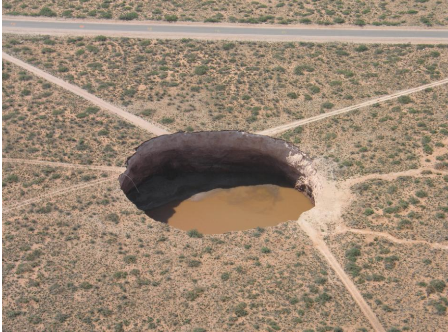
Figure 4: JWS sinkhole on 7/19/2008, three days after initial catastrophic collapse. Water in sink is ~12 m below ground level. View to south, with County Road 217 in background.
