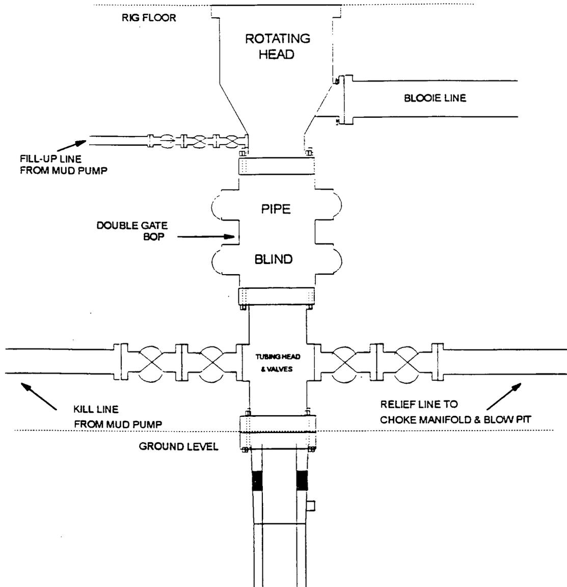
Minimum BOP installation for Completion operations. 7 1/16" Bore (6" Nominal), 2,000 psi minimum working pressure double gate BOP to be equipped with blind and pipe rams.
