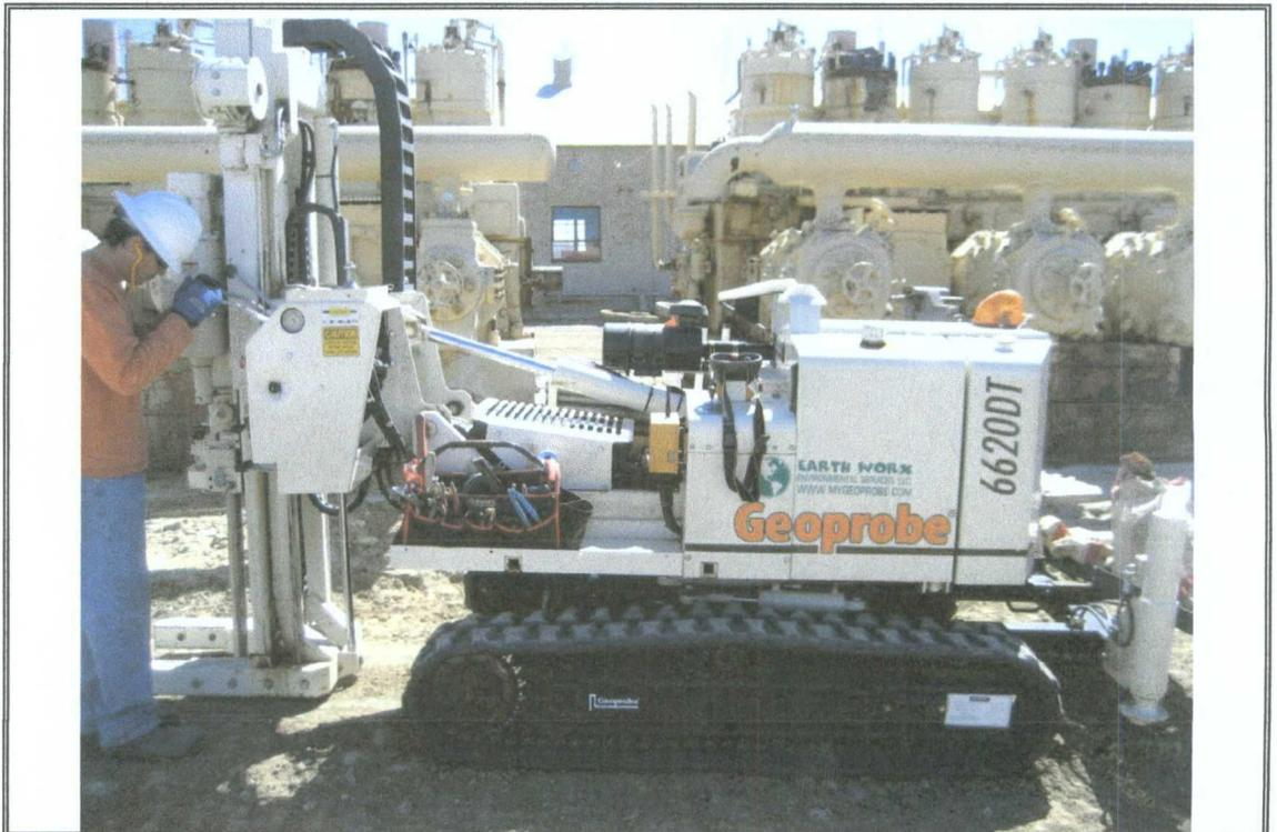
Photograph Number 2: View of the geoprobe direct push unit performing borings on the west side of the former Clark compressor building.
