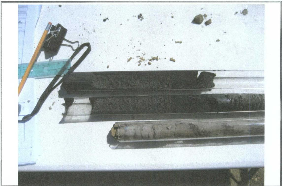
Photograph Number 6: View of black hydrocarbon contaminated soils encountered at soil boring SB7W at a depth of eight (8) feet below ground surface.
