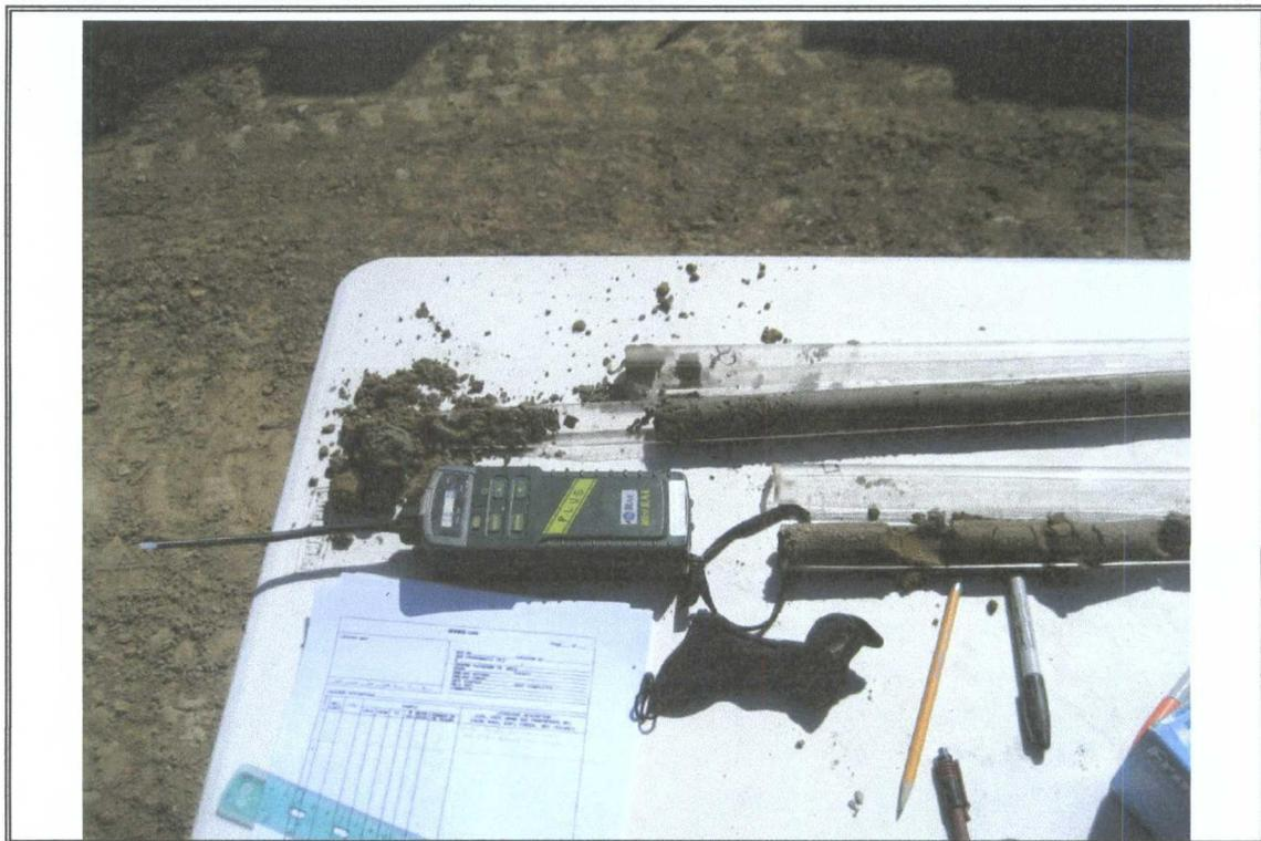
Photograph Number 3: View of soils collected in a polycarbonate liner in the process of field screening.
