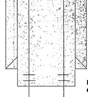
12 ¼" Hole; 8 5/8" Csg. Set @ 374'. Cemented w/200 Sx. Cement circulated to surface.
