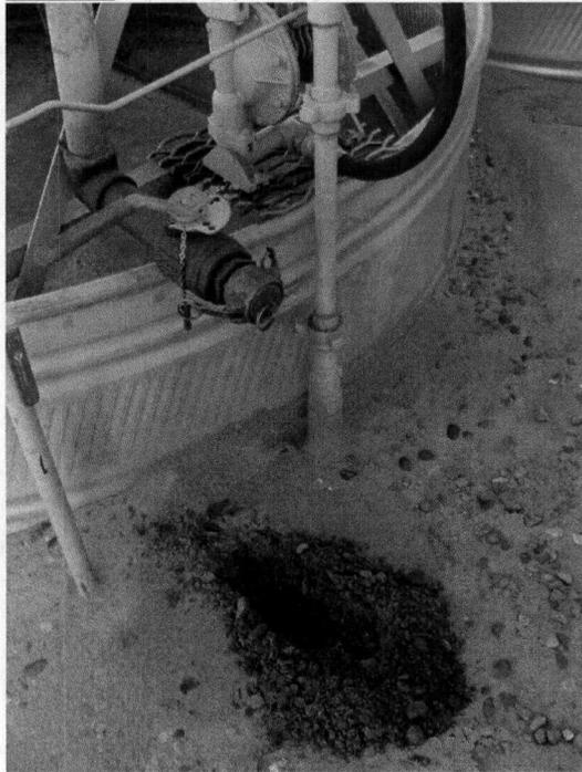
Photo 7: Saddle tank area with discharge conduit outside of secondary containment. Soil staining.
