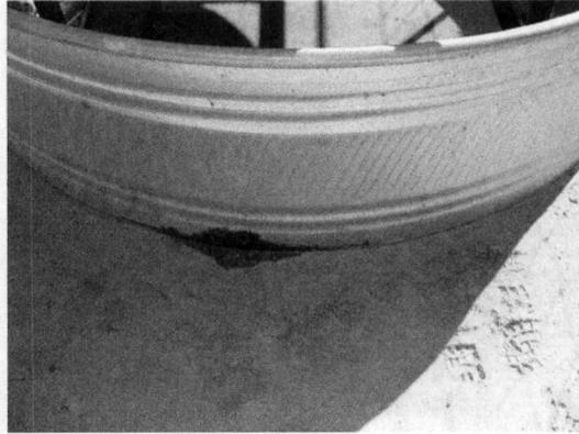
Photo 4: Leak at bottom of secondary container. Holding fluids.
