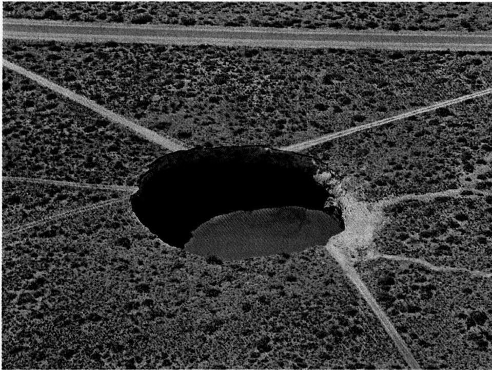
**Figure 4:** Loco Hills Sinkhole #1 on 7/19/2008, three days after initial catastrophic collapse. Water in sink is ~12 m below ground level. View to south, with County Road 217 in background.
