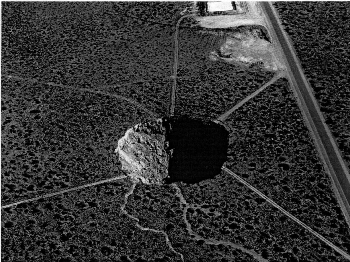
**Figure 8:** Loco Hills Sinkhole #1 on 11/18/2008. Note continued presence of concentric fractures. Boulders visible on left flank of sinkhole are approximately car-size.
