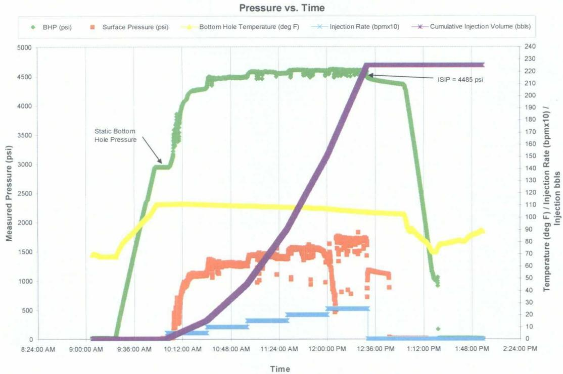
In conclusion, we feel that this step-rate test successfully determined the actual formation parting pressure of the subject Delaware reservoir and is equal to 4485 psi bottomhole and 1547 psi surface. Therefore, Fasken Oil and Ranch, Ltd. request that the maximum allowable surface injection pressure for the Ling Federal No. 1 be raised from 1135 psi to 1547 psi.
