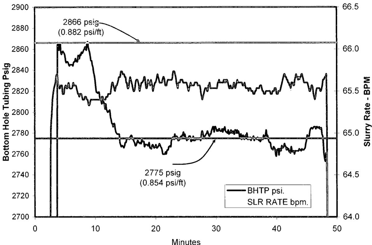
Figures 1 and 2, above, were generated using the same data from the March 1, 1996 Postfrac Treatment Summary. Figure 1 depicts the pressure and slurry rate versus time. To enhance detail, Figure 2 has a larger scale than Figure 1. These figures show the following:
