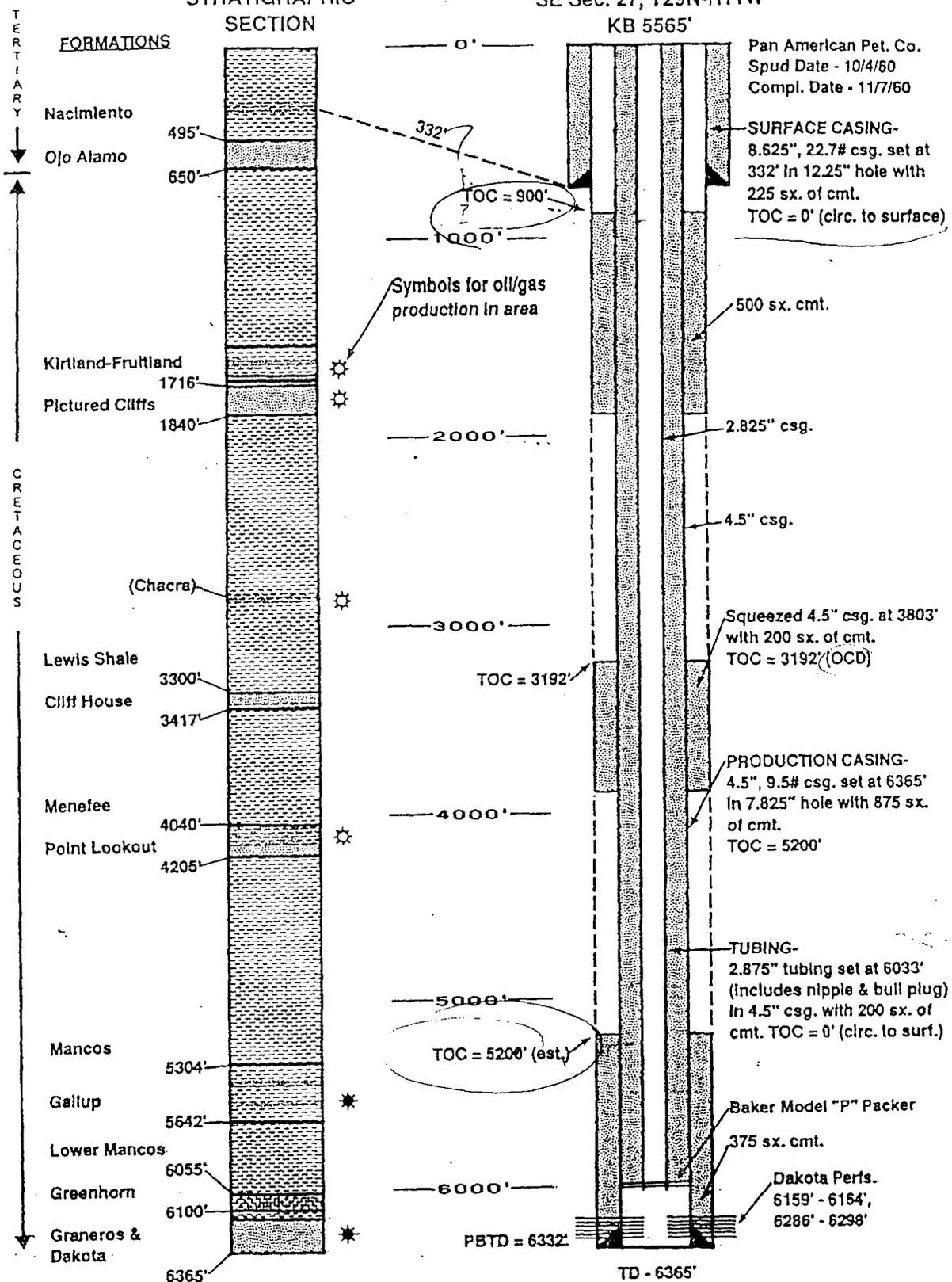
Figure 3. Wellbore diagram of the present day Amoco Davis Gas Com "F" No. 1 well and corresponding stratigraphy. Producing zones in the immediate area are also shown along the stratigraphic column.
