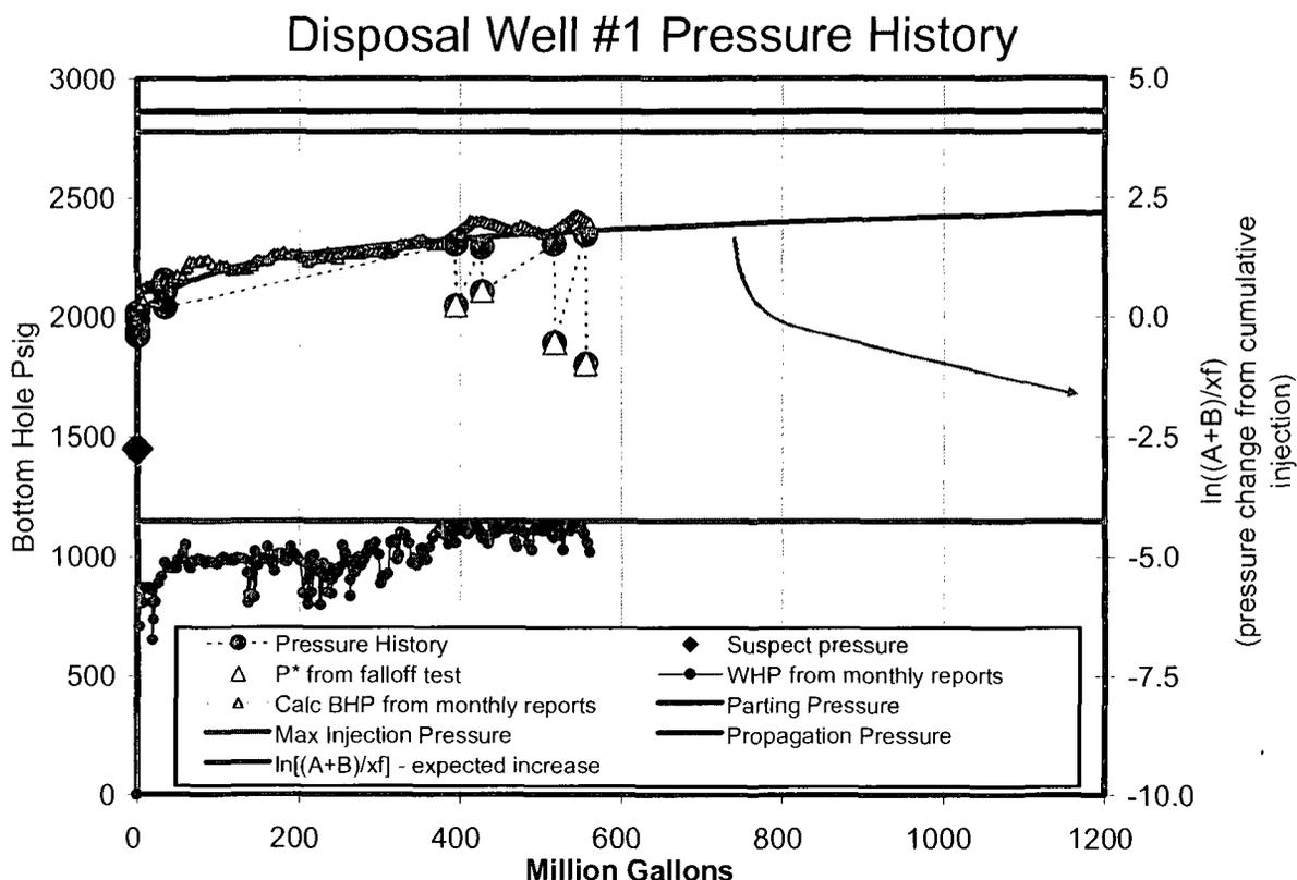
Figure 3, above, depicts bottom hole pressure and injection pressure history versus cumulative injection volume from initiation of injection to near present. The figure also depicts the formation pressure change from cumulative injection (black line), formation parting pressure (red line), propagation pressure (green) and permitted maximum injection pressure (blue line).
