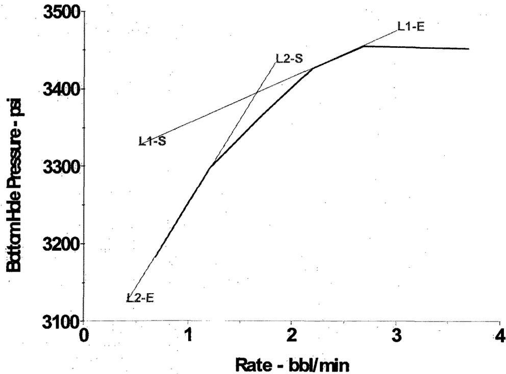
Lines L1-S & L2-S are based upon the inflection point of the rate vs. bottom hole pressure curve. The point of intersection defines the estimated fracture parting pressure, 3389 psi.
